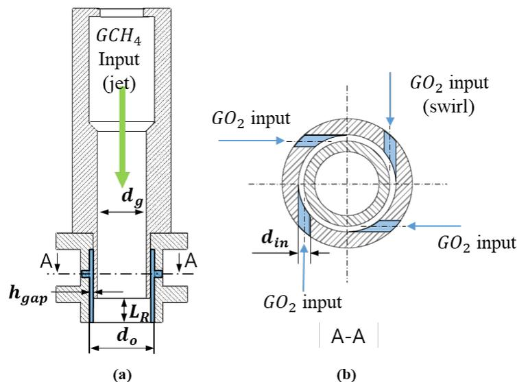
Figure 2: The design parameters: (a) near the injector exit and (b) the  $GO_2$  tangential swirl hole
