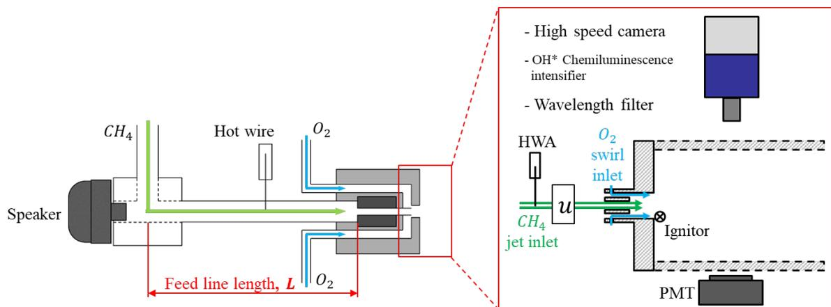
Figure 1: Schematics of jet-swirl  $GCH_4-GO_2$  model injector and  $OH^*$  signal measurement devices (high speed camera and PhotoMultiplier Tube, PMT)
