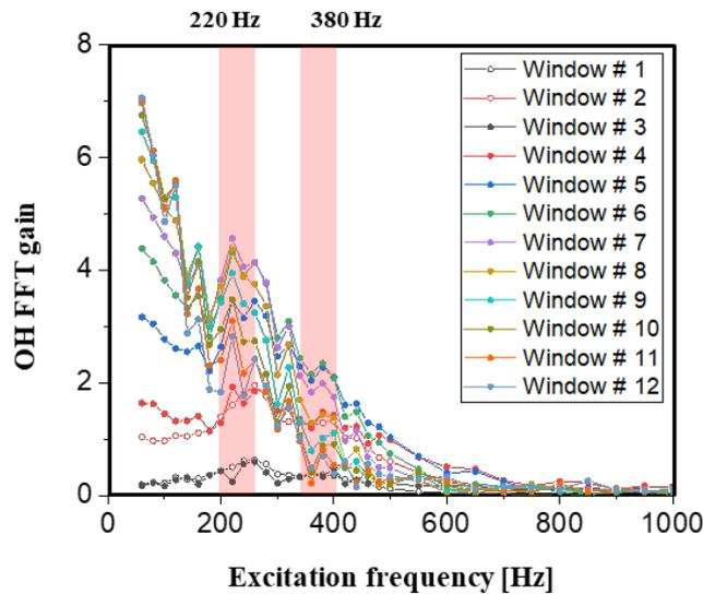
Figure 4: Acoustic response of flame to perturbation frequencies along interest windows
