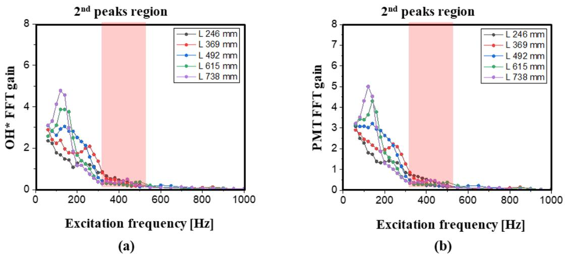
Figure 5: The entire flame signal response along excitation frequencies, (a) OH\* chemiluminescence signal of overall window and (b) the PMT signal.
