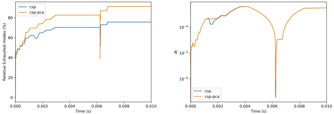
Figure 3: Relative number of exhausted modes  $M$  (left) and integration time-step (right) in function of time for the full CSP case (blue) and the reduced CSP-PCA model (orange).
