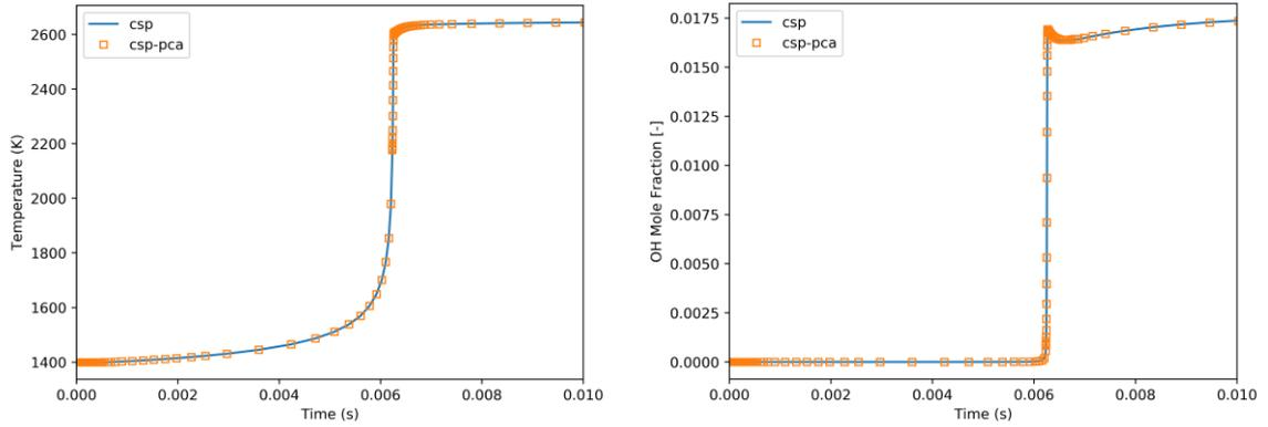
Figure 2: Temperature (left) and  $OH$  model fraction (right) in function of time for the full CSP case (line) and the reduced CSP-PCA model (symbols).
