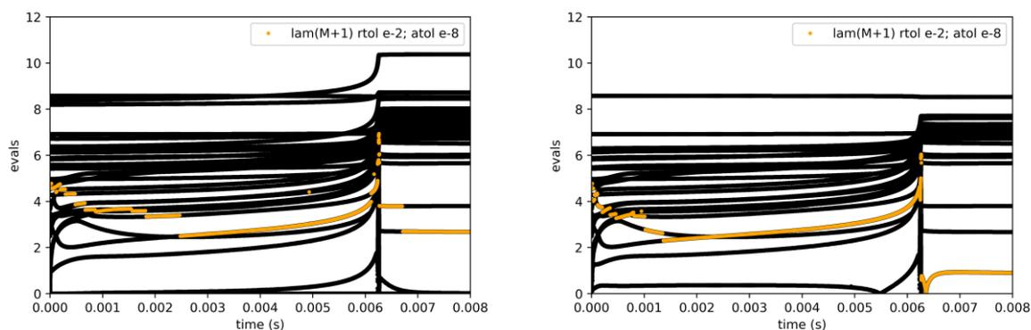
Figure 1: Eigenvalues (black) and  $(M + 1)$ -th eigenvalue (orange) against time for the detailed CSP (left) and reduced CSP-PCA (right) systems.
