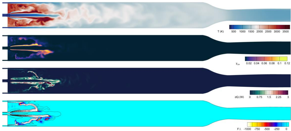
Fig. 3 Temperature, OH mass fraction, heat release rate, and the Takeno flame index distribution in the lateral slice. The solid line in the flame index contour indicates the value of zero and the dashed line indicates the negative values of the flame index.
