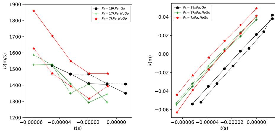
Figure 7: The evolution of the velocity of the shock (left) and the travelled distance by shock over time (right) in the mixture CH<sub>4</sub>/2O<sub>2</sub> at T<sub>0</sub>=293 K. In all cases, the solid lines are along the top wall and the dashed lines are along the bottom wall of the shock tube.
