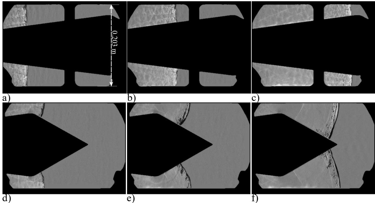
Figure 3: The formation of the overdriven detonation through converging channel (a, b, c) and the decay of the shocks in the diverging channel (d, e, f) in  $\text{CH}_4/2\text{O}_2$  mixture at the initial temperature of 293 K and the initial pressure of 17 kPa.
