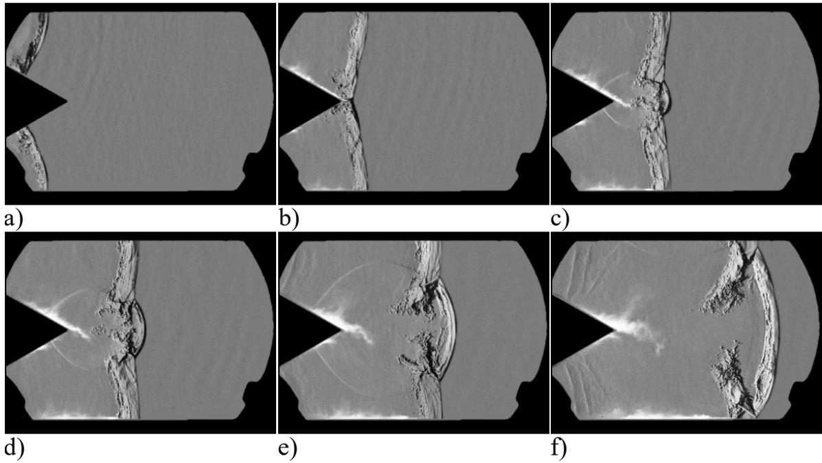
Figure 4: The formation of a decaying Mach shock in CH<sub>4</sub>/2O<sub>2</sub> mixture at an initial temperature and pressure of 293K and 17 kPa, respectively.
