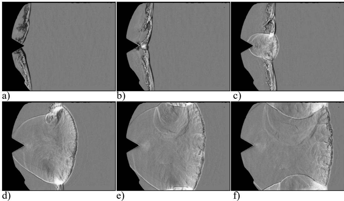
Figure 5: The formation of a detonative Mach shock in CH<sub>4</sub>/2O<sub>2</sub> mixture at an initial temperature and pressure of 293K and 17 kPa.
