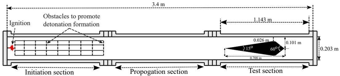
Figure 2: Schematic of the shock tube used in the experiments.
