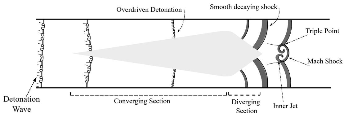
Figure 1: Schematic of the experimental configuration to isolate a reactive Mach reflection.
