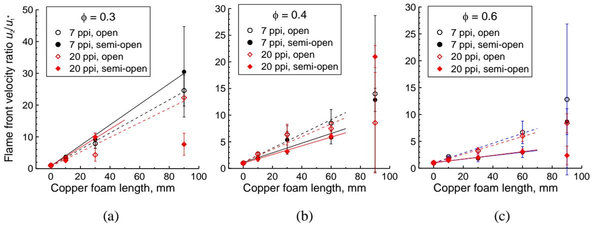
Figure 4: Flame front velocity ratios  $u_2/u_2^*$  for hydrogen-air mixture with (a)  $\phi = 0.3$ , (b)  $\phi = 0.4$  and (c)  $\phi = 0.6$ .
