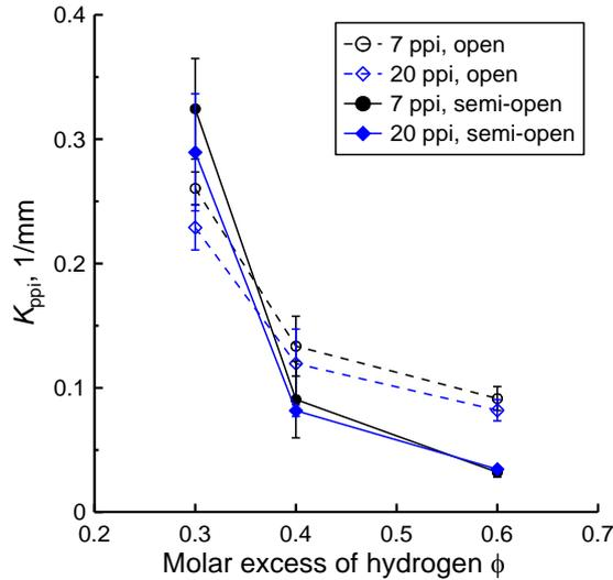
Figure 5: Dependence of effectiveness  $K_{\text{ppi}}$ , on molar excess  $\phi$  of hydrogen. Solid lines/filled symbols – semi-open channel; dashed lines/empty symbols – open channel.
