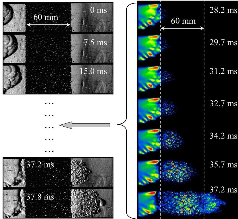
Figure 2: Sequential schlieren and IR images of the flame front in hydrogen-air mixture when passing through the copper foam, 7 ppi, length 60 mm.  $\phi = 0.3$ . The first image is taken as the zero time moment.
