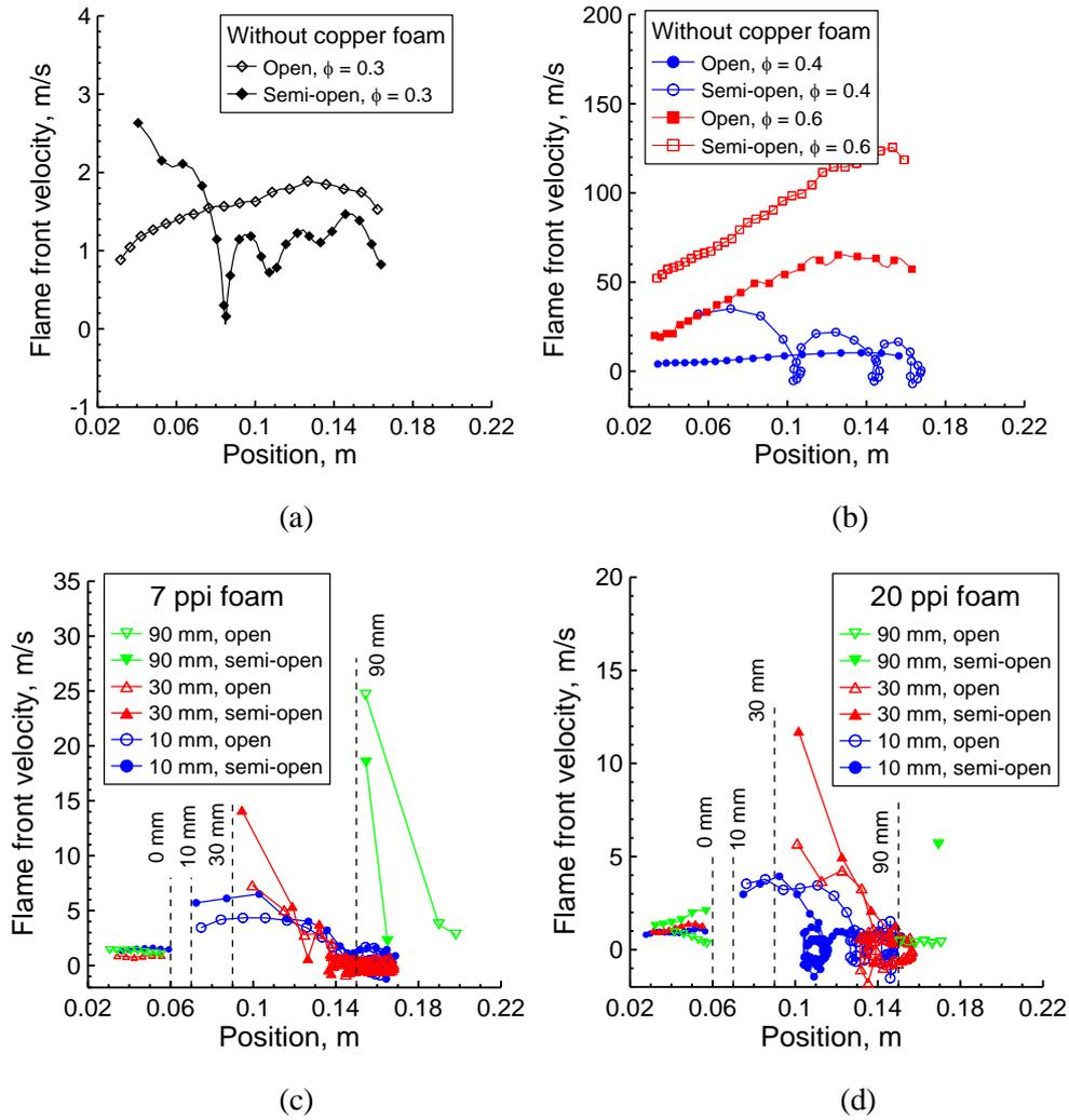
Figure 3: Flame front velocity in hydrogen-air mixture in diagnostic section (a) without porous copper,  $\phi = 0.3$ , (b) without porous copper,  $\phi = 0.4, 0.6$ , (c) with 7 ppi copper foam,  $\phi = 0.3$ , (d) with 20 ppi copper foam  $\phi = 0.3$ . The distance is given from the beginning of the diagnostic section.
