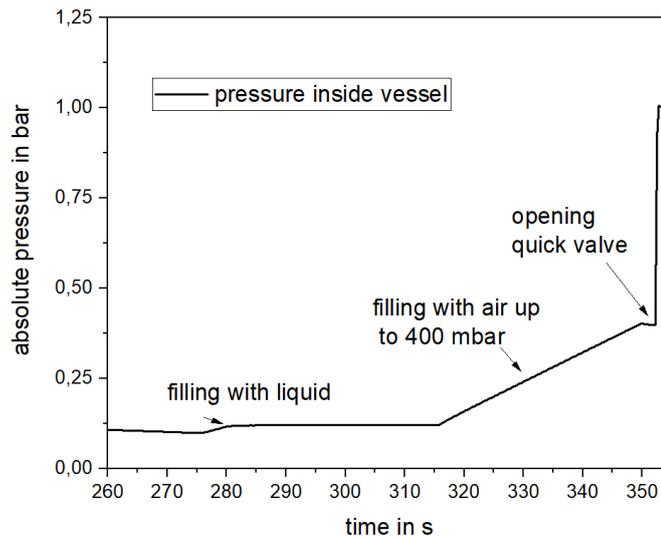
**Fig 2: Absolute pressure during experiment in the 20L-Sphere**
