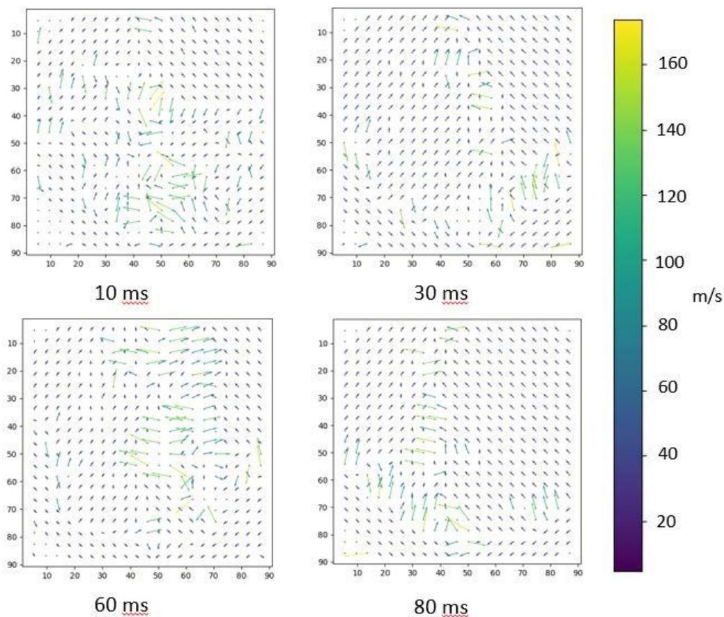
Fig 5: Selected frames of the dispersion within the test mixture with phosphorescence particles and their streamlines analysed with OpenPIV
