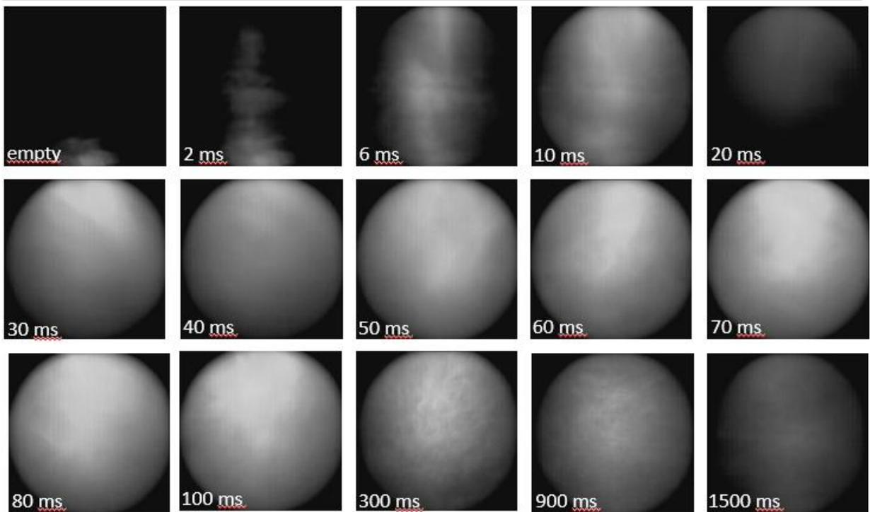
*Fig 3: Selected frames showing hybrid dispersion with 2 vol% acetone and 125 g/m<sup>3</sup> corn starch with 2 % titanium dioxide tracers*
