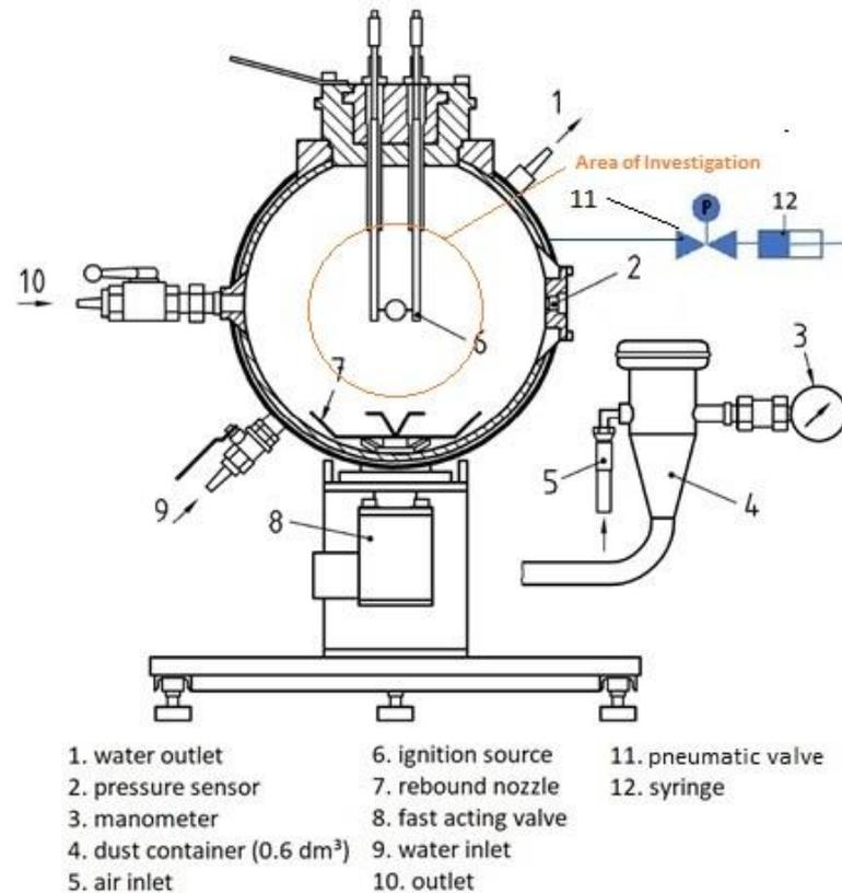
*Fig 1: Schematic experimental setup*
