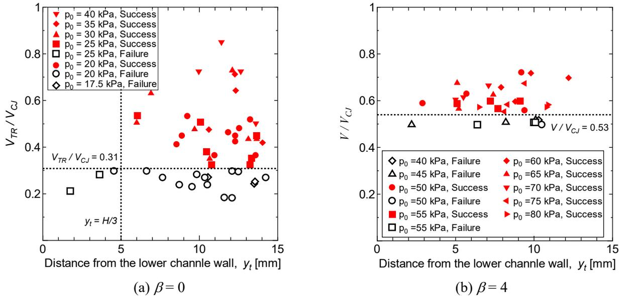
Figure 4: Wave velocities in detonation diffraction for  $\text{C}_2\text{H}_4 + 3\text{O}_2 + \beta\text{Ar}$ .  $V_{TR}$ : velocity of transvers wave,  $V$ : velocity of quenched detonation wave just before onset of explosion.
