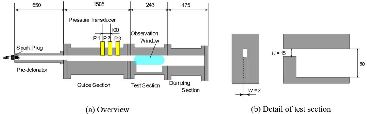
Figure 1: Schematics of experimental apparatus for diffraction and re-initiation of detonation.
