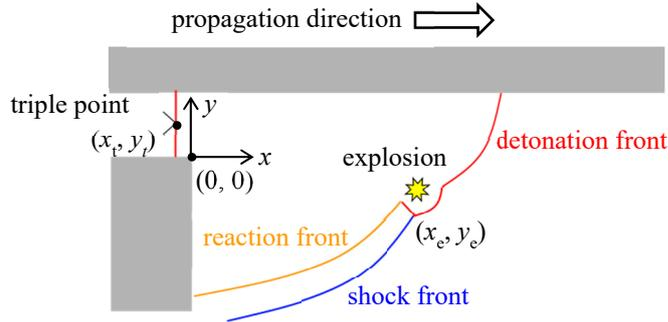
Figure 3: Coordinate system to analyze detonation diffraction. Depicted waves show the case of detonation re-initiation for  $\beta = 4$ .
