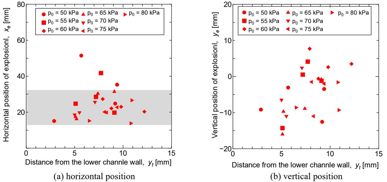
Figure 5: Relationship between explosion location ( $x_e, y_e$ ) and triple point position from the lower channel wall  $y_t$  in detonation diffraction for  $C_2H_4 + 3O_2 + 4Ar$ .
