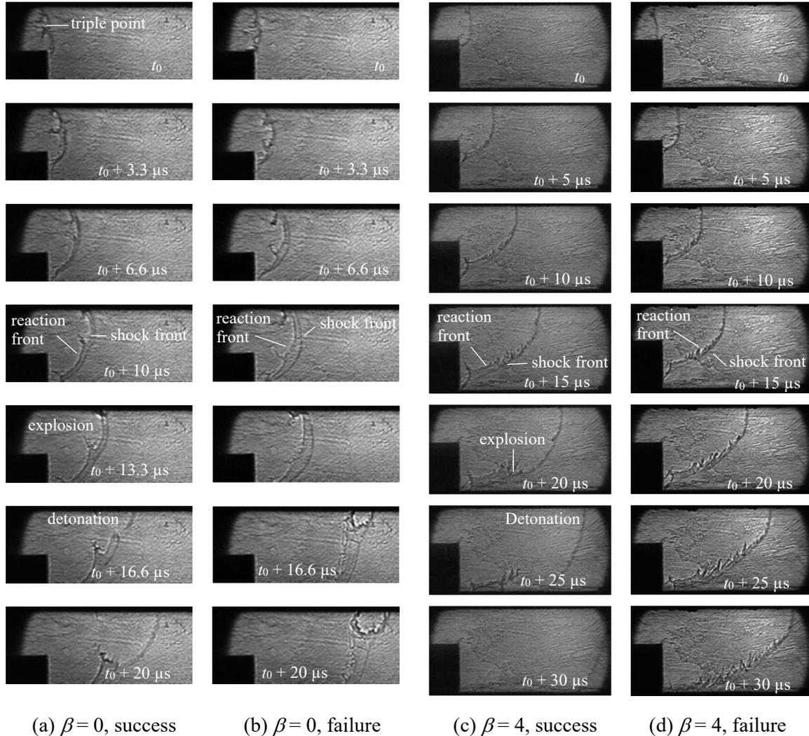
Figure 2: High-speed shadowgraph images of detonation diffraction for  $C_2H_4 + 3O_2 + \beta Ar$ .  $\beta=0$  and  $p_0=20\text{kPa}$  for (a) and (b),  $\beta=4$  and  $p_0=50\text{kPa}$  for (c) and (d).
