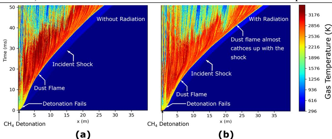
Figure 2: X-t diagram for the 40-m long channel with  $30\ \mu\text{m}$  particles shaded by gas phase temperature at  $y = 5\ \text{cm}$  (a) without radiation and (b) with radiation.
