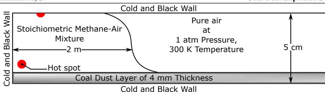
Figure 1: Initial and boundary conditions of the numerical setup.
