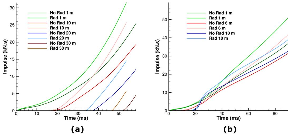
Figure 5: Impulse plots for the (a) 40-m channel at locations of 1 m, 10 m, 20 m and 30 m; and (b) 10-m channel at locations of 1 m, 6 m and 10 m in the channel, and at a height of 2.5 cm in the channel. Both radiative and non-radiative cases with 30  $\mu\text{m}$  particles are shown.
