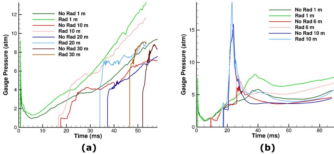
Figure 4: Gauge pressure plots for the (a) 40-m channel at locations of 1 m, 10 m, 20 m and 30 m; and (b) 10-m channel at locations of 1 m, 6 m and 10 m in the channel, and at a height of 2.5 cm in the channel. Both radiative and non-radiative cases with 30  $\mu\text{m}$  particles are shown.
