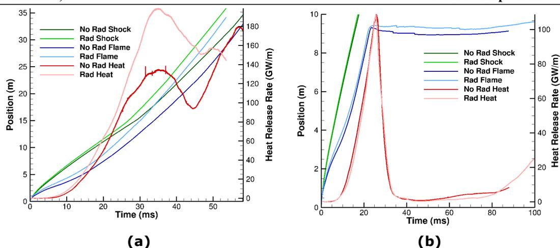
Figure 3: Shock and flame positions and heat release rates due to chemical reactions with  $30\ \mu\text{m}$  particles for the (a) 40-m channel and (b) 10-m channel.
