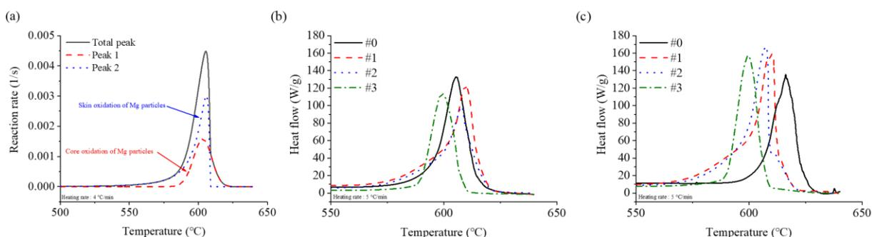
Figure 3: DSC results (a) Peak separation of pristine mg particle at 4 °C/min (b) 5 °C/min and 50 ml/min (c) 5 °C/min and 100 ml/min
