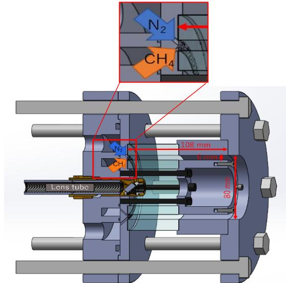
Figure 1: Schematic of RDE combustor
