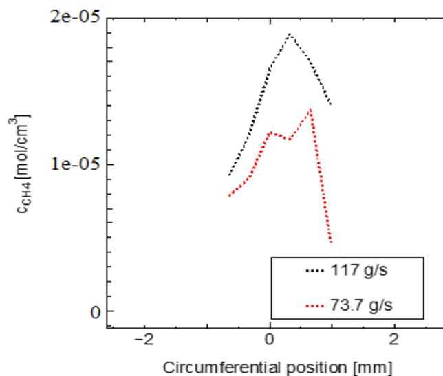
Figure 7: Fuel concentration distribution in the combustion condition
