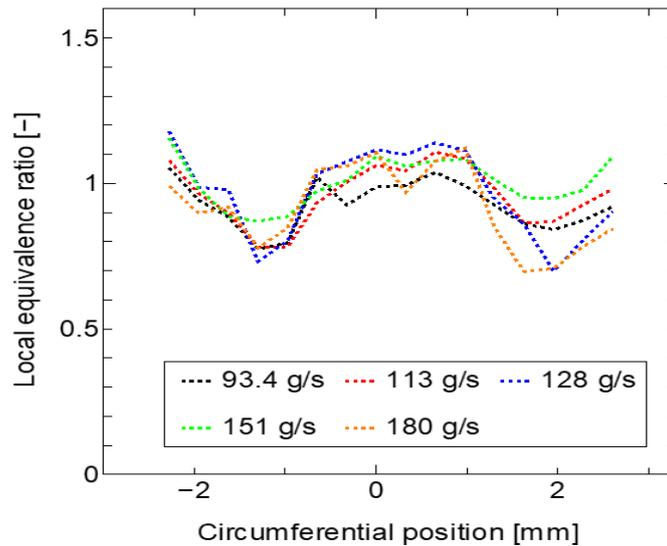
Figure 5: Local equivalence ratio for various mass flow rates.
