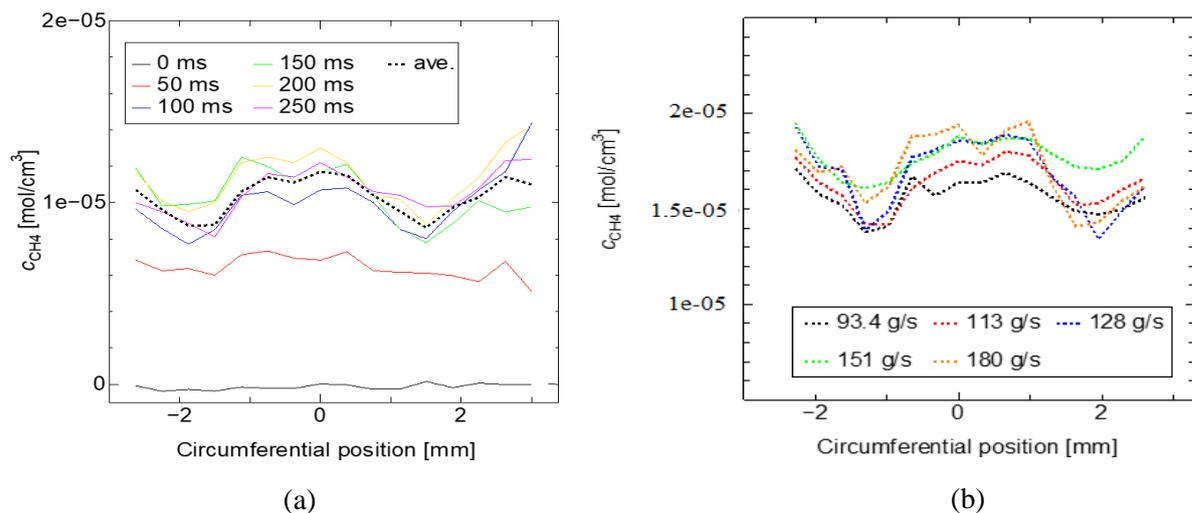
Figure 4: a) Time changes of fuel concentration  $\dot{m}_{CH_4} = 36.9$  g/s distribution  $\dot{m}_{N_2} = 178$  g/s; b) Fuel concentration distribution for various mass flow rate.
