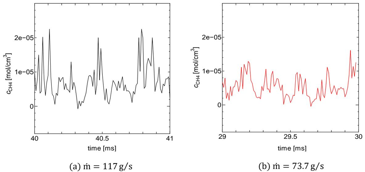
Figure 6: Fuel concentration histories in the combustion chamber.
