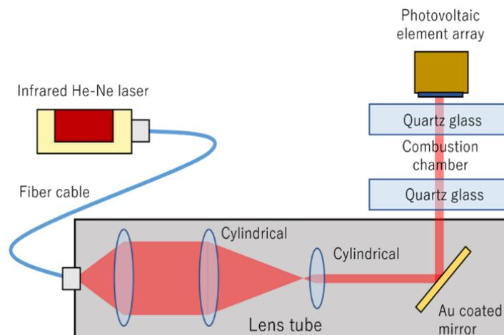
Figure 2: Optical setup of laser extinction method
