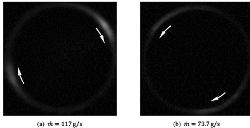
Figure 8: The captured image of detonation propagation
