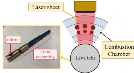
Figure 3: Measurement method of the fuel concentration distribution
