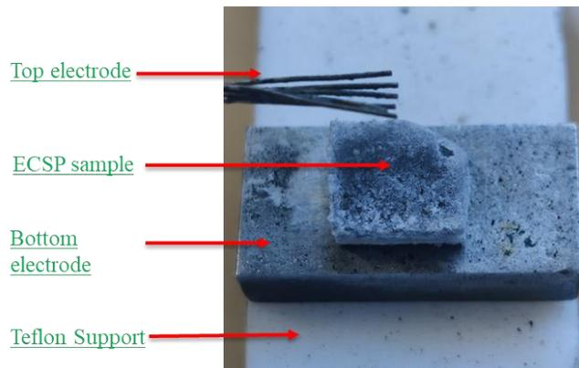
Figure 2: Setup with nichrome wire as one electrode.
