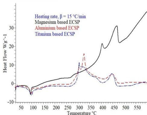
Figure 2: DSC curve for Mg, Al and Ti based ECSP at heating rate of 15 °C/min
