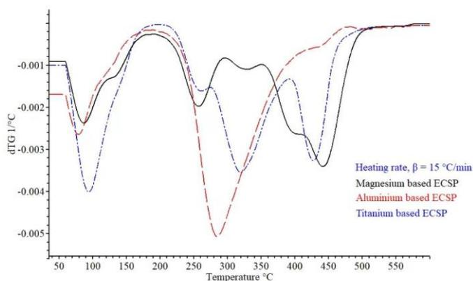
Figure 4: dTG curve for Mg, Al and Ti based ECSP at heating rate of 15 °C/min.
