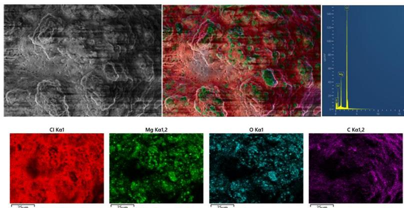
Figure 1: SEM image and EDS mapping of residues from thermal experiments for Mg based composition.
