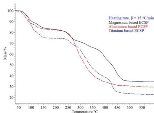
Figure 3: TGA curve for Mg, Al and Ti based ECSP at heating rate of 15 °C/min.
