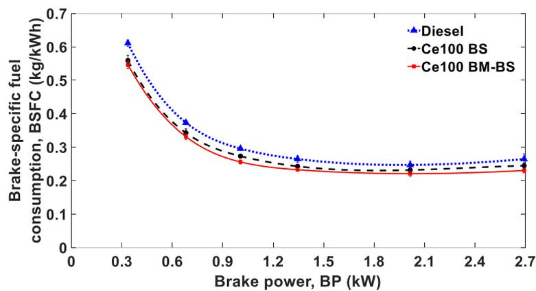
Figure 2: Brake-specific fuel consumption (BSFC) of the VCR engine (@ 1100 RPM, CR=20).
