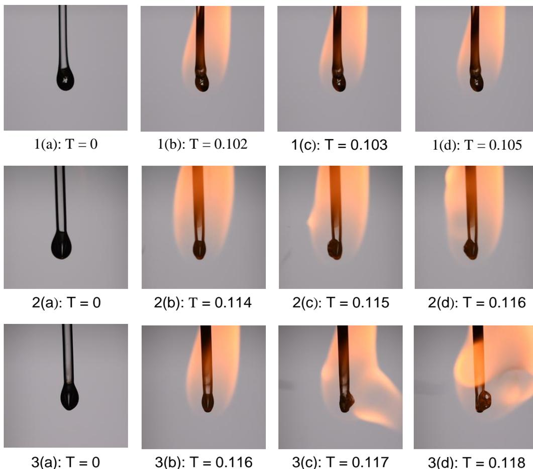
Figure 4: Droplet evaporation images for the following fuel samples: (1) Diesel, (2) Ce100 BS, and (3) Ce100 BM-BS; the event of micro-explosion in case of nanofuel [ $T = t/D_0^2$ , 't' is in seconds, 'D<sub>0</sub>' is in mm, and 'T' is in sec/mm<sup>2</sup>]
