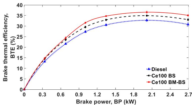
Figure 3: Brake thermal efficiency (BTE) of the VCR engine (@ 1100 RPM, CR=20).
