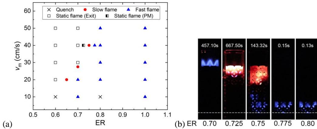
Fig. 2 (a) Flame propagation modes under different inlet conditions, (b) Flame photographs at  $v_m = 40$  cm/s.
