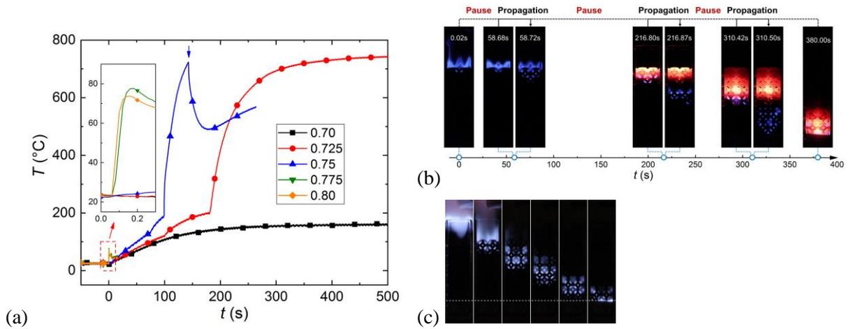
Fig. 3 (a) Temporal temperature curves of TC7 at  $v_m = 40$  cm/s. (b) Propagation process of slow flame at  $ER = 0.70$  and  $v_m = 27.5$  cm/s. (c) Propagation process of fast flame at  $ER = 1.00$  and  $v_m = 30.0$  cm/s.
