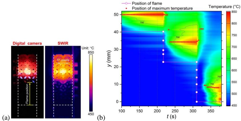
Fig. 4 (a) Slow flame position and temperature distribution at  $t = 300$ s; (b) Temporal evolution of the flame position and the temperature distribution.
