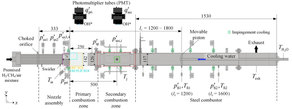
Figure 1: Cross-sectional view of an axial-fuel-staged lean-premixed combustor composed of four sections.  $p_i$  and  $T_i$  indicate dynamic pressure transducers and type-K thermocouples. Abbreviations: us = upstream, pri = primary, tp = transition piece, sec = secondary, ft = flame tube, exh = exhaust section. Dimensions in millimeters.
