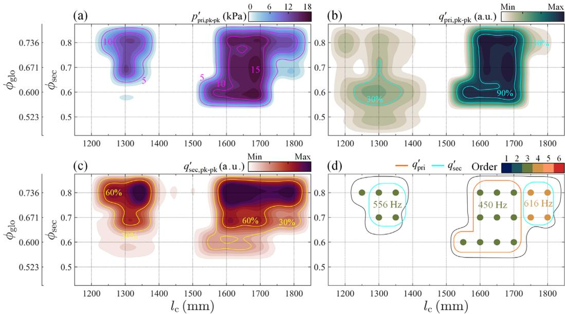
Figure 2: Stability maps plotted as a function of equivalence ratio of the secondary combustor and combustor length; cutoff amplitude for pressure perturbations is set to 1.0 kPa (peak-to-peak). (a) peak-to-peak pressure fluctuation amplitude. Magenta numbers indicate pressure amplitude of selected iso-contours (unit: kPa). (b, c) Peak-to-peak heat release rate oscillation intensities from both combustion chamber. (d) Orders of longitudinal modes calculated from FEM-based Helmholtz simulations.
