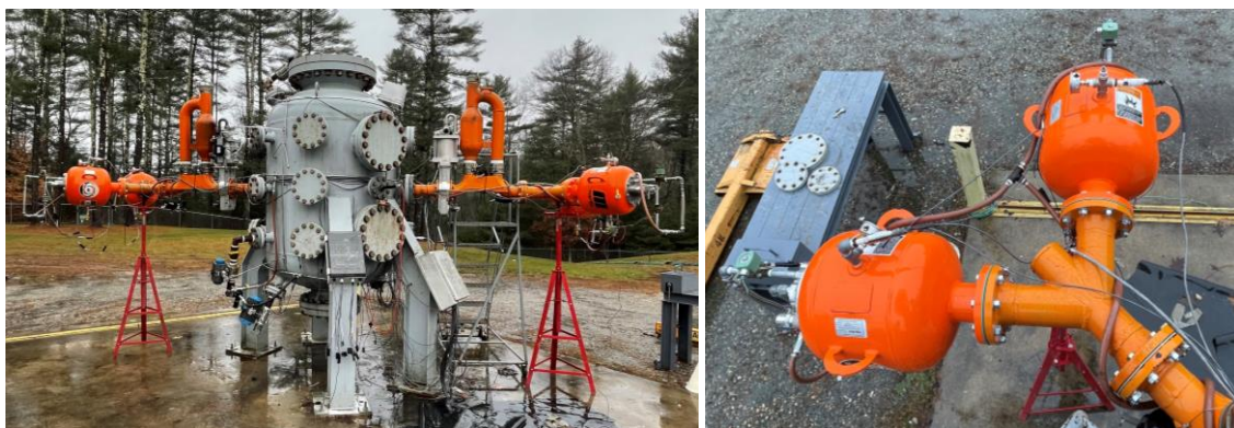
Figure 1: An image of the 2.5-m 3 test vessel setup showing both dust injectors (left) as well as an image of the dual air cannon configuration (right).
