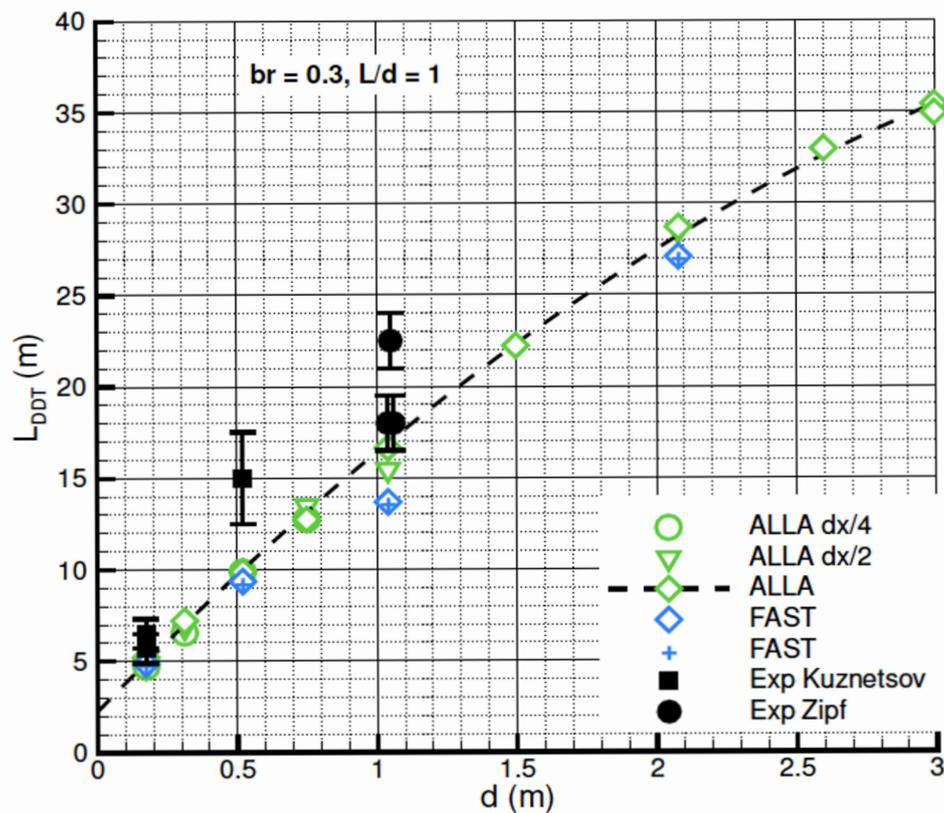
Figure 3: A collection of computed and measured distances to DDT as a function of channel height  $d$  for stoichiometric methane-air mixture. References and more details are given in [6].
