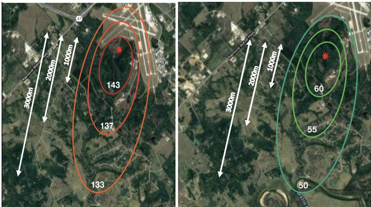
Figure 2: Extent of noise levels (in db) caused by detonation exiting the DRTF. Left: Unmitigated. Right: With muffler. For comparisons, 140 db is the pain threshold, 80 db is the level 30 m from a freight train, and 60 db is a conversation at 1 m.
