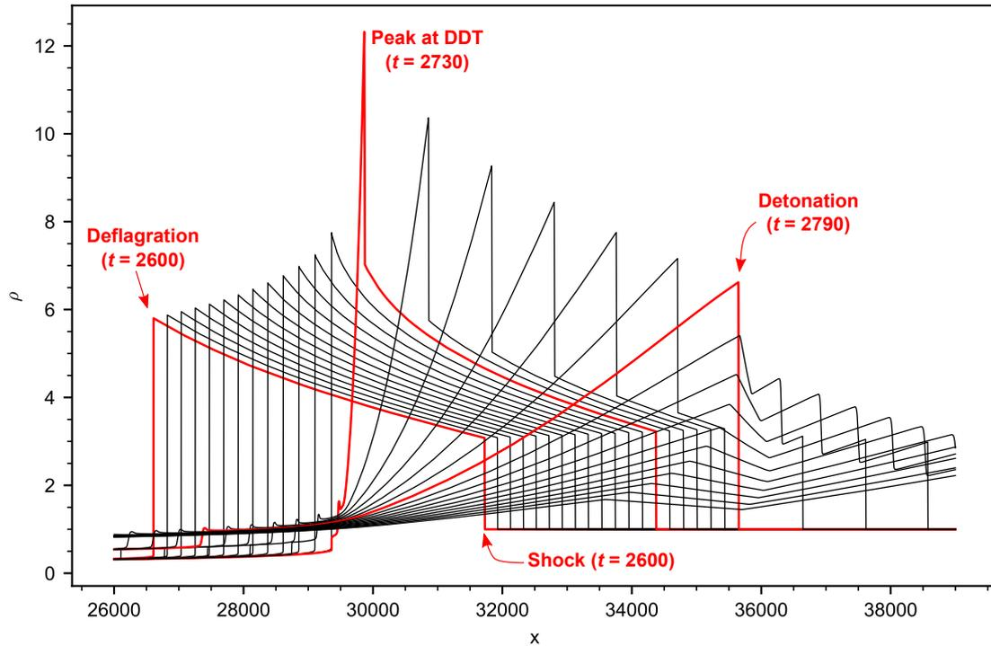
Figure 2: Series of density profiles plotted around the time of transition to detonation (see Figure 1(b)). Time interval between each plot is 10.
