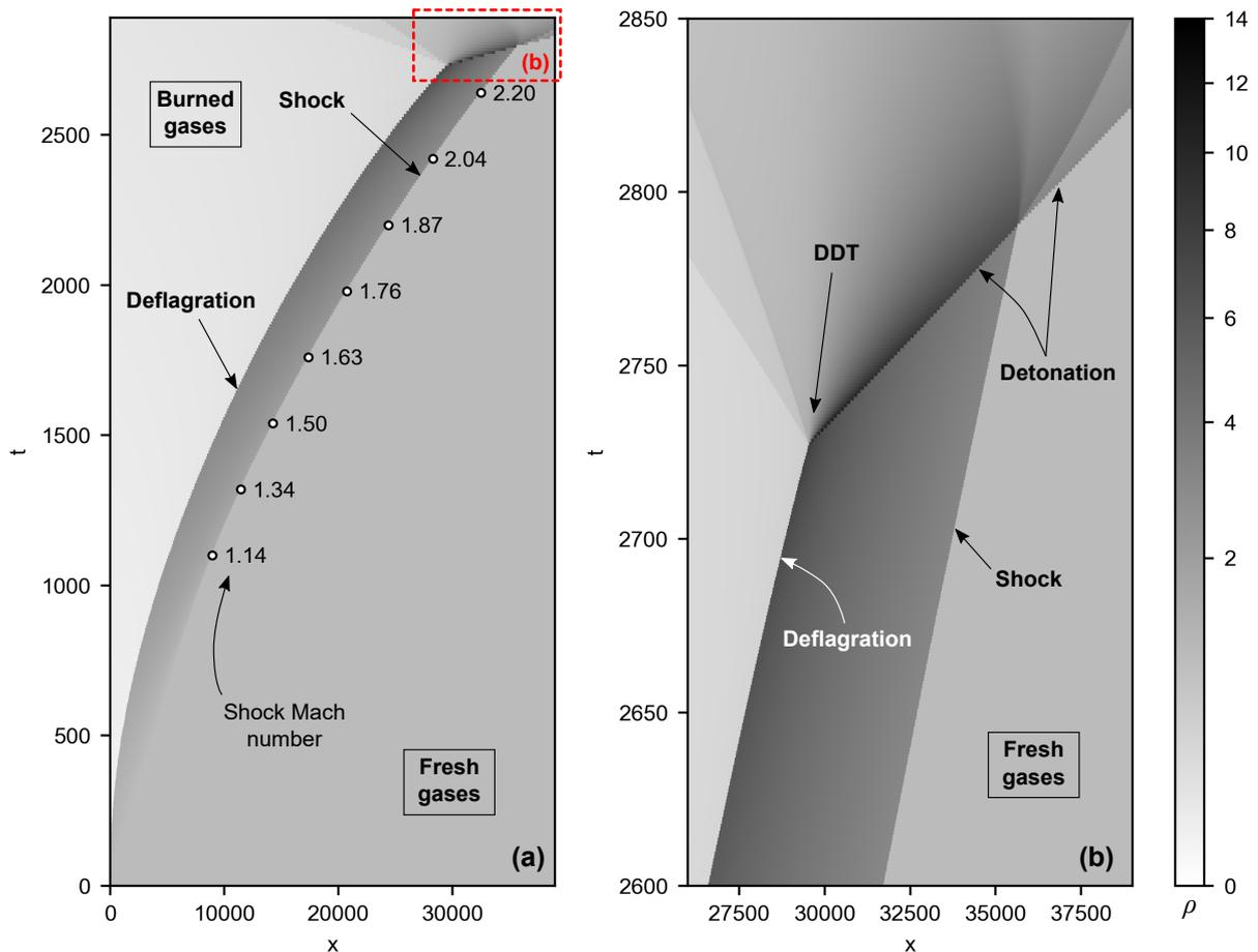
Figure 1: Space-time diagram plotted for density of the flame acceleration process. (a) shows the overall evolution of the flame and the shock, which strength is annotated along its trajectory. (b) shows the late stages of the flame acceleration process, where transition to detonation occurs.
