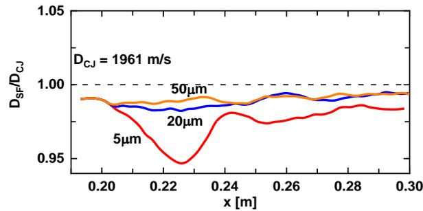
Figure 2: Influence of the particle diameter on the shock speeds of hydrogen detonation wave, scaled by the C—J value of pure gas mixture.  $c = 1 \text{ kg/m}^3$ .
