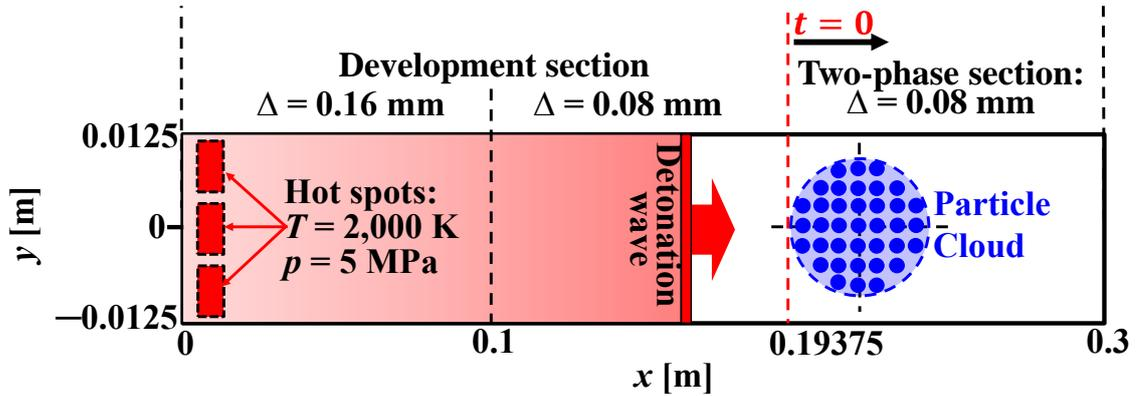
Figure 1: Schematic of the computational domain. The blue dots represent particles. Domain and particle sizes not to scale.
