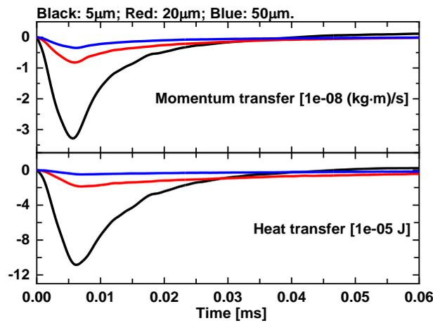
Figure 3: Influence of the particle diameter on the interphase transfer of momentum and heat.  $c = 1 \text{ kg/m}^3$ .
