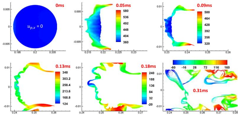
Figure 4: Time history of particle cloud morphology.  $c = 1 \text{ kg/m}^3$  and  $d_p = 5 \mu\text{m}$ . Axis label unit: m.
