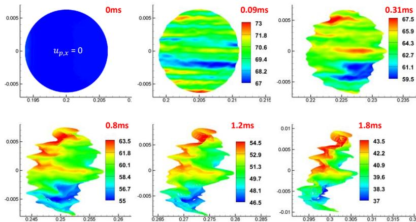
Figure 5: Time history of particle cloud morphology.  $c = 1 \text{ kg/m}^3$  and  $d_p = 50 \mu\text{m}$ . Axis label unit: m.
