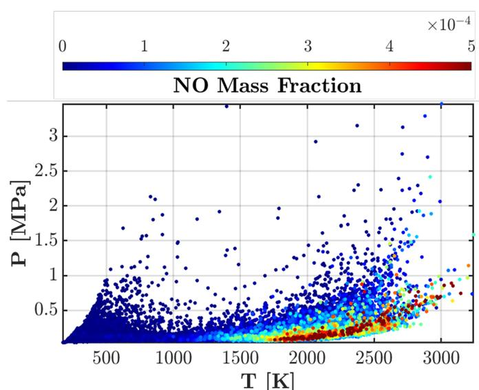
Figure 3: Pressure vs temperature colored by corresponding NO mass fraction for all particle measurements.
