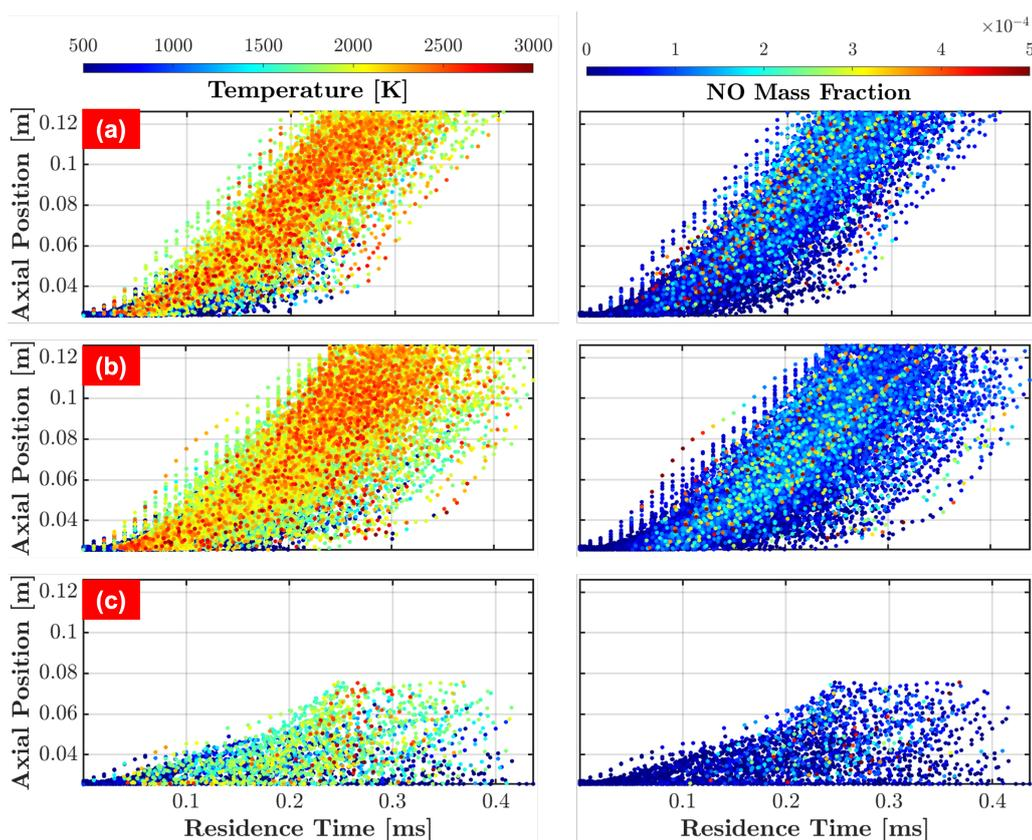
Figure 2: Temperature and NO mass fraction for particles experiencing at least 1 full cycle of residence time (0.24 ms) divided into particles that have (a) axially reached the exit plane of the combustor, (b) axially reached between the midpoint and exit plane of the combustor, and (c) did not axially reach the midpoint of the combustor.
