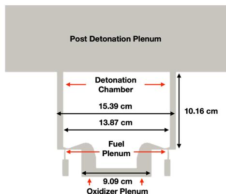
Figure 1: Cross-section schematic of AFRL RAI RDE configuration.
