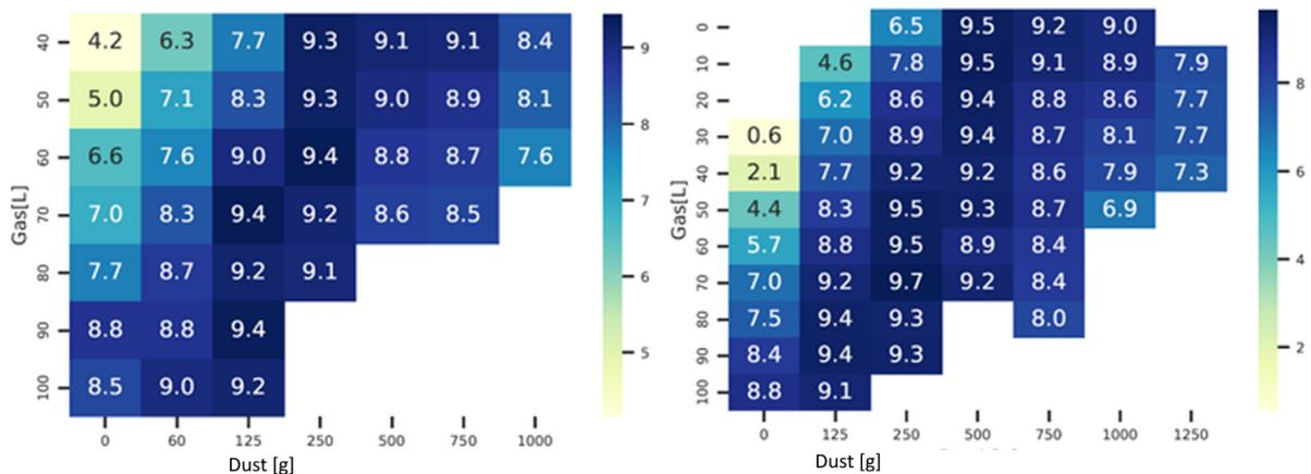
Figure 2: hybrid maximum explosions pressure in the 1 m<sup>3</sup> vessel for 2 kJ (left) and 10 kJ (right) ignition energy.
