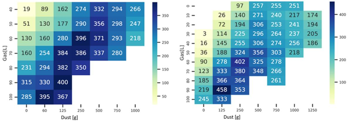
Figure 3: hybrid maximum pressure rise velocity in the 1 m<sup>3</sup> vessel for 2 kJ (left) and 10 kJ (right) ignition energy.
