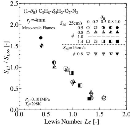
Fig.4 Relationships between  $S_L/S_{L\infty}$  at  $r_f=4$ mm and  $Le$  for mixtures with  $S_{L0}=25$ & $15$ cm/s
