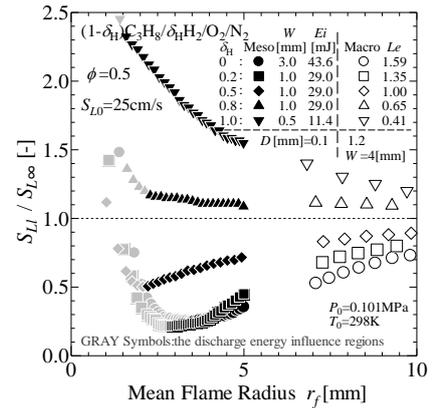
Fig.2 Relationship between  $r_f$  and  $S_{Li}/S_{L\infty}$  ( $\phi=0.5$ ,  $S_{L0}=25\text{cm/s}$ )
