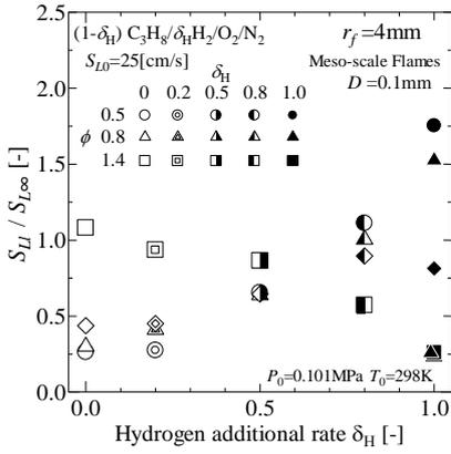
Fig.3 Influences of  $\phi$  and  $\delta_H$  on  $S_L/S_{L\infty}$  at  $r_f=4$ mm for mixtures with  $S_{L0}=25$ cm/s
