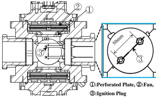
Fig.1 Schematic of combustion chamber for turbulence.
