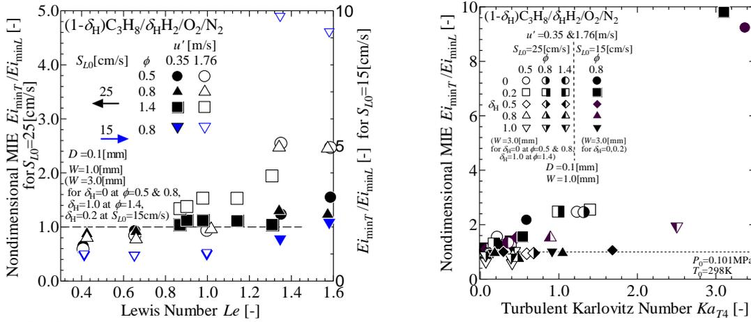
Fig. 7 Relationships between  $Ei_{minT}/Ei_{minL}$  and  $Le$  for mixtures with  $S_{LO}=25$  &  $15$  cm/sFig. 8 Relationship between  $Ka_{T4}$  and  $Ei_{minT}/Ei_{minL}$  as functions of  $\phi$ ,  $\delta_H$  and  $u'/S_{LO}$
