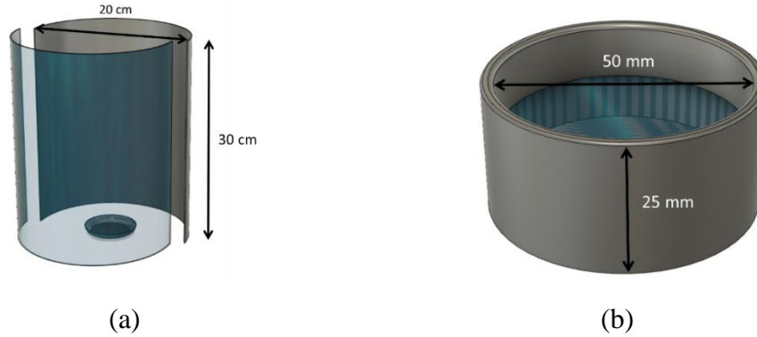
Figure 2. (a) Physical structure of two half-cylindrical walls of the fire whirl boundary. (b) Size of the fuel pool that is being utilized to generate the fire whirl.
