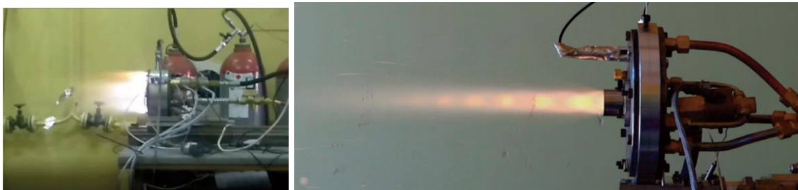
Figure 2: Rocket engines with detonation combustion chambers supplied by \text{N}_2\text{O} and \text{C}_3\text{H}_8 - with annular cylindrical detonation chamber and aerospike nozzle (left) and with disc-shape detonation chamber and bell nozzle (right).
