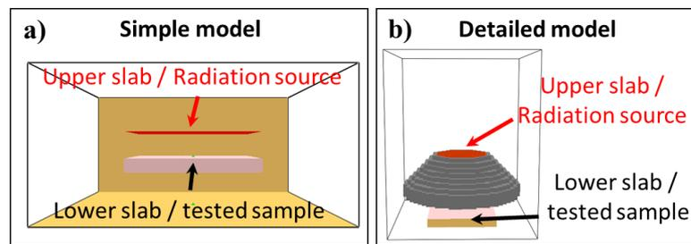
Figure 3. Representation of the CC radiation source: a) simple model; b) detailed model.
