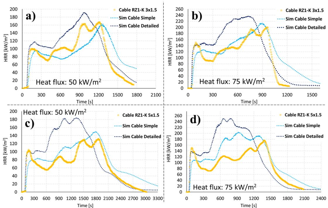
Figure 4. HRR curves for CC tests to cables and simulations curves: a) RZ1-K  $3 \times 1,5 \text{ mm}^2$  cable at  $50 \text{ kW/m}^2$ ; b) RZ1-K  $3 \times 1,5 \text{ mm}^2$  cable at  $75 \text{ kW/m}^2$  pieces; c) RZ1-K  $5 \times 1,5 \text{ mm}^2$  cable at  $50 \text{ kW/m}^2$ ; d) RZ1-K  $5 \times 1,5 \text{ mm}^2$  cable at  $75 \text{ kW/m}^2$ .
