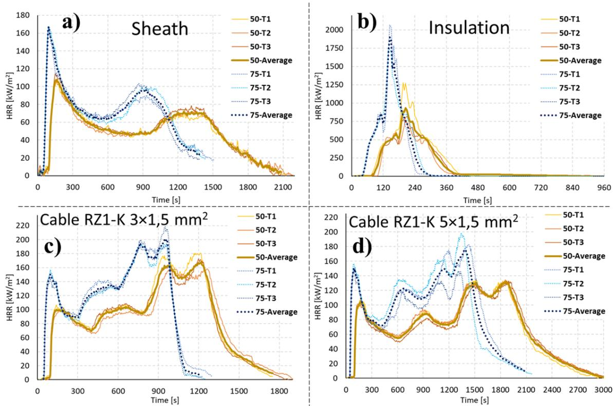
Figure 1. HRR curves for CC tests carried out: a) sheath element; b) insulation element; c) RZ1-K  $3 \times 1,5 \text{ mm}^2$  cables (10 pieces); d) RZ1-K  $5 \times 1,5 \text{ mm}^2$  cables (8 pieces).
