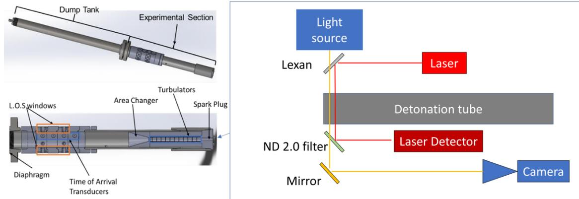
Figure 1: Schematic Diagram of *UCF*'s detonation tube (left) and optical setup (right).
