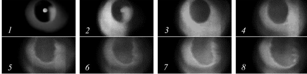
Figure 4: Series of photographs obtained with the Photron SA-Z 2100K high-speed camera, the frame spacing  $5.55 \times 10^{-6}$  s,  $We = 1.92 \times 10^6$  (diameter = 6.8 mm). DW travels from left to right with a CJ velocity = 2337.6 m/s.
