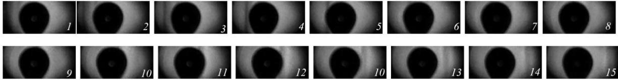
Figure 5: High-speed images of a shock wave crossing a fuel droplet (diameter = 5.8 mm) obtained with the Photron SA-Z 2100K high-speed camera, the frame spacing  $0.83 \times 10^{-6}$  s,  $We = 230 \times 10^3$  (wave travels from left to right with a velocity = 900 m/s).
