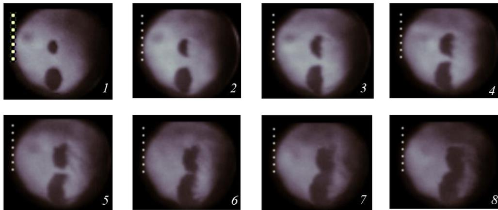
Figure 3: Series of photographs obtained with the Phantom Miro M310 high-speed camera, the frame spacing  $2.94 * 10^{-6}$  s,  $We = 359 * 10^3$  for top droplet (diameter = 1.2 mm) and  $We = 666 * 10^3$  for bottom droplet (diameter = 2.3 mm). DW travels from left to right with a CJ velocity=2391.2 m/s.
