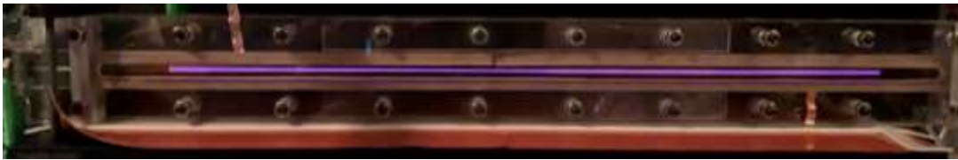
Figure 1: Image of ns-DBD plasma generated in the cell.
