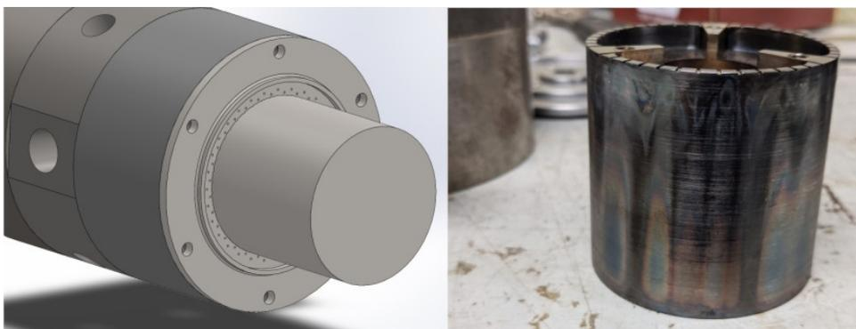
Figure 2: Model of the RDE with face injectors shown without the outer combustion chamber wall (left). Note the location of the radial injection slots, along the injector plate surface in the central part (right).
