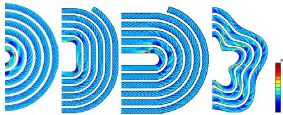
Fig. 1 Numerical smoked-foil records of detonation wave propagations in various cross-sections.
