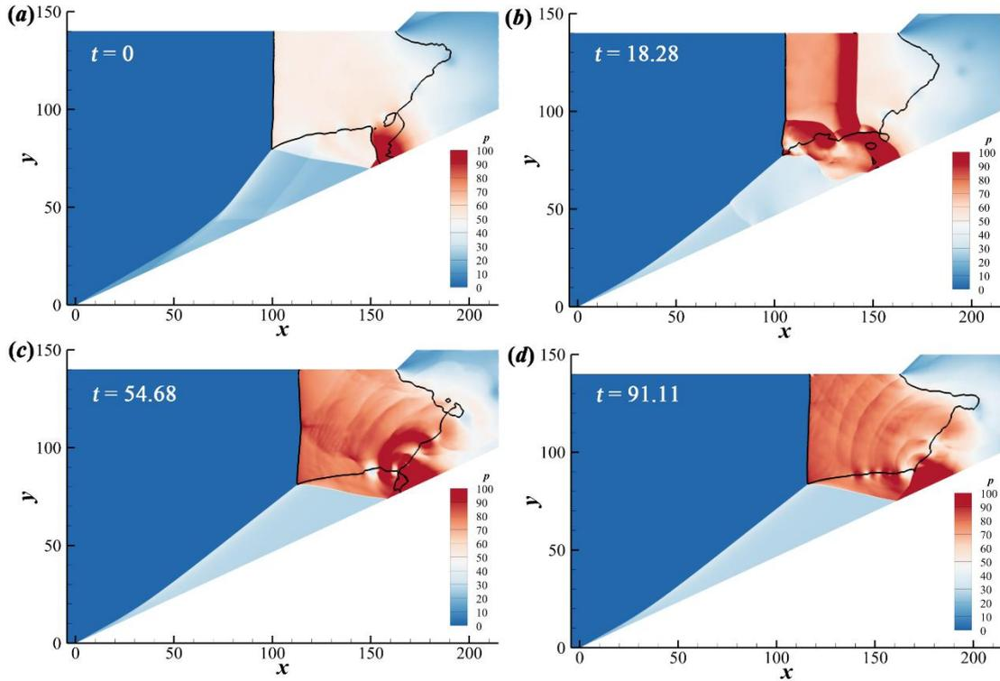
Figure 5: Pressure field for evolution of  $Ma$  7.0 to 9.0 based on position 2; The black line denotes the subsonic zone.
