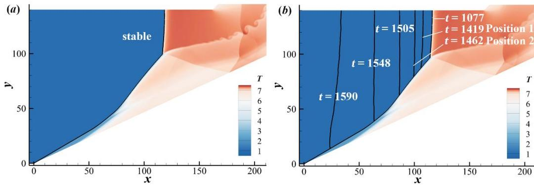
Figure 2: Temperature field for stable with  $L_c = 162$ (a), unstable with  $L_c = 163$ (b). The black lines represent the position of leading shock wave front.
