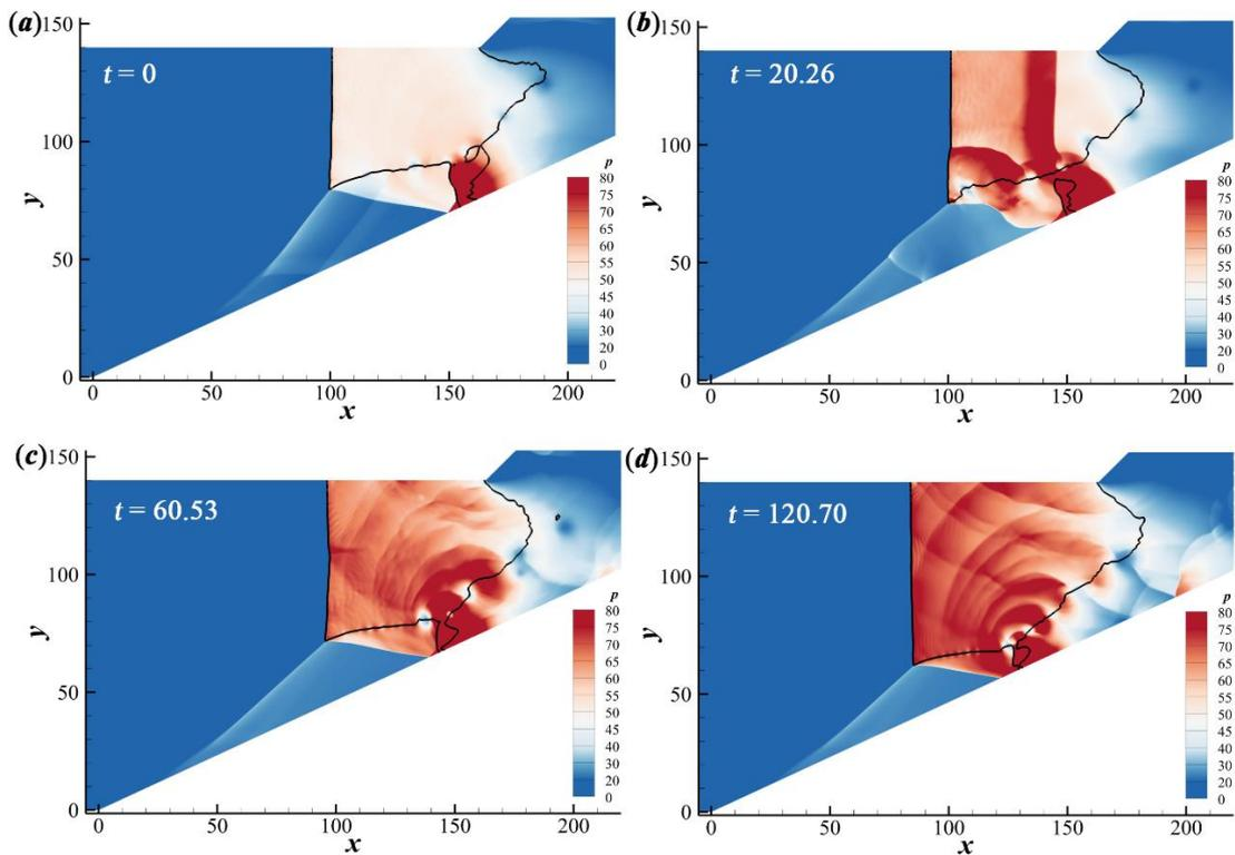
Figure 4: Pressure field for evolution of  $Ma$  7.0 to 8.0 based on position 2 The black line denotes the subsonic zone.
