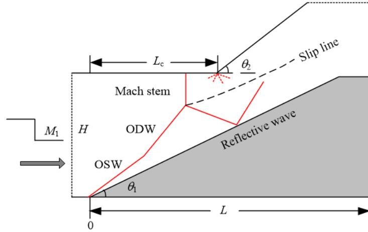
Figure 1: The schematic of the domain for combustor.
