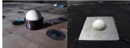
Figure 2: 42g (IRSN facility) and 333g (ISL Facility) Hexomax® charges
