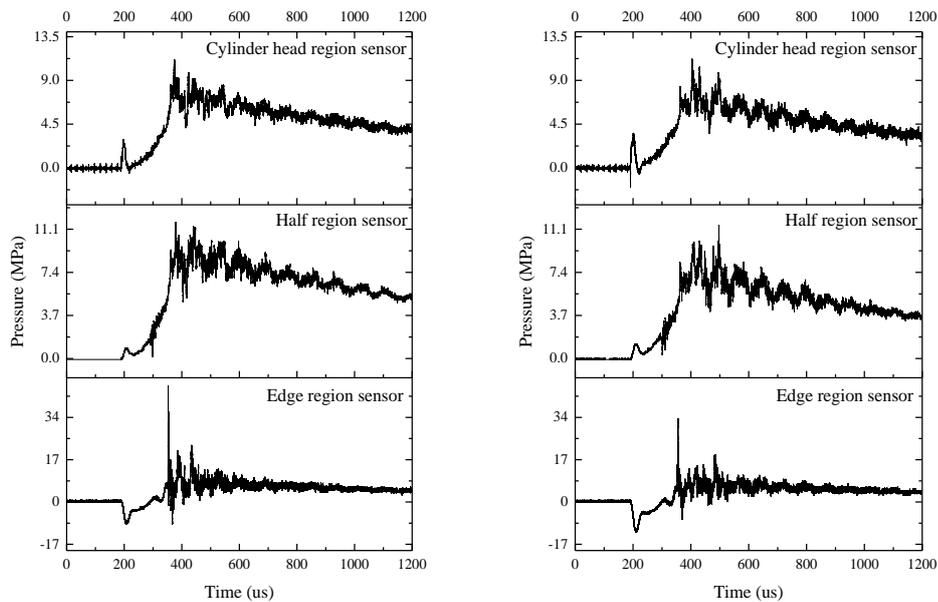
(a) Low ignition energy experimental results (b) High ignition energy experimental results
