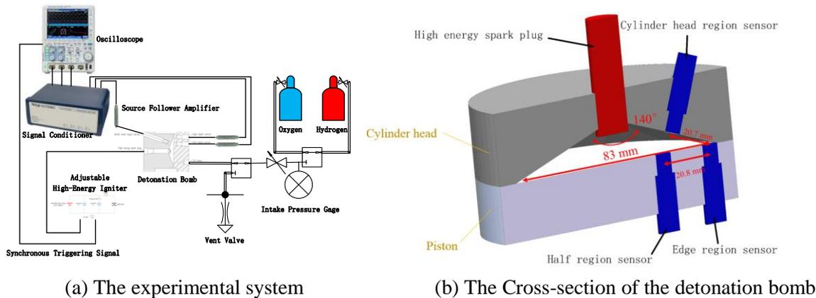
Figure 1: The system of the detonation bomb device.
