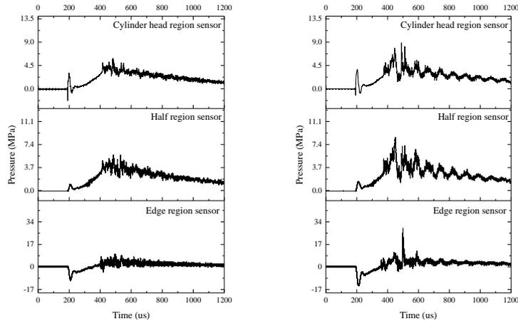
(a) Low ignition energy experimental results      (b) High ignition energy experimental results
