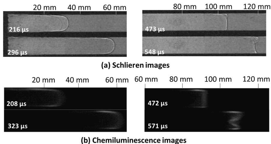
Figure 4: Schlieren and chemiluminescence images in the smooth wall condition
