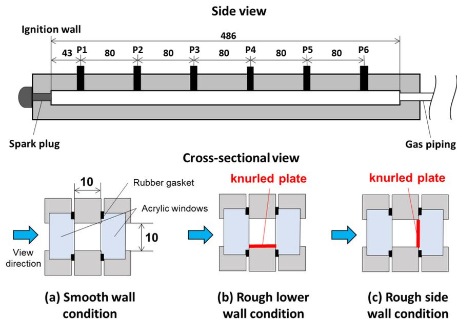
Figure 1: Experimental apparatus (unit of length: mm).
