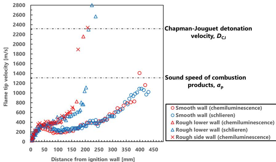
Figure 3: Evolutions of the flame tip velocity in the schlieren and chemiluminescence observations in each wall condition.
