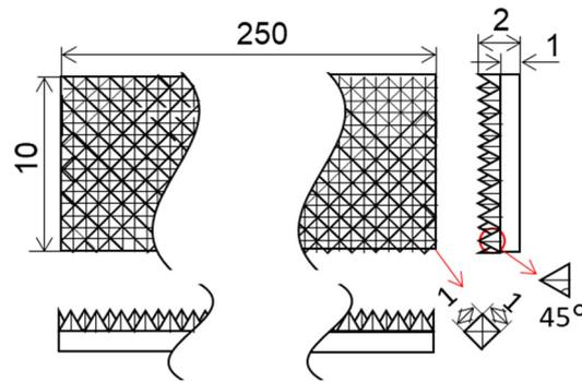
Figure 2: Stainless-steel plate with knurling (unit of length: mm).
