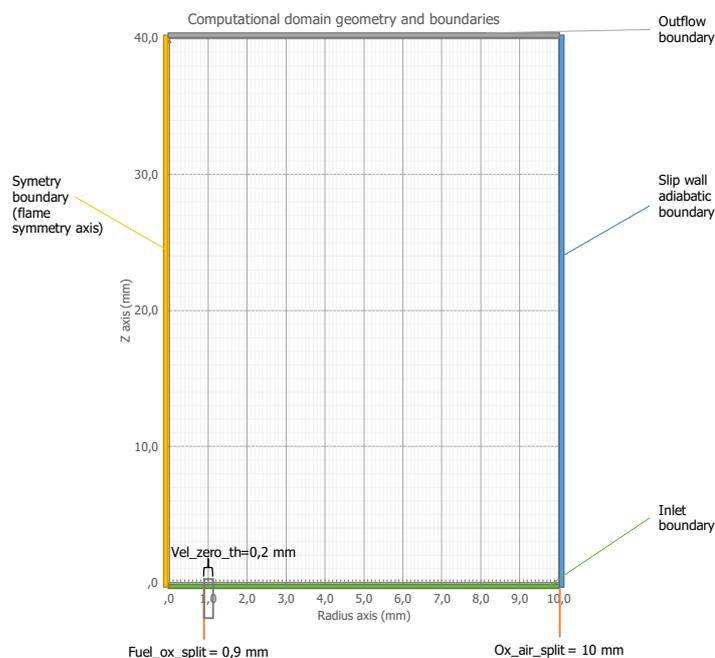
Figure 1: Computational domain geometry and boundary conditions.
