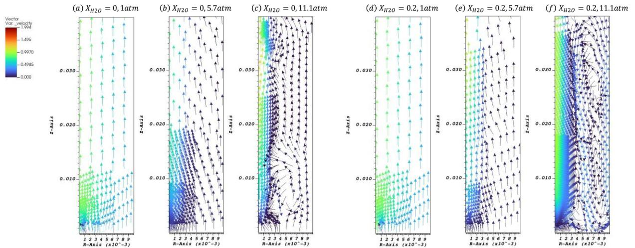
Figure 4: Simulated flame velocity profiles at 1, 5.7, and 11.1 atm with 0%, (a) – (c) and 20%, (d) - (f) water mole addition: The vector length only represents the direction.
