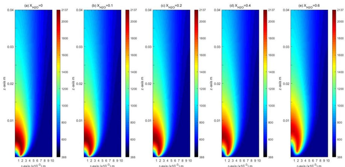
Figure 2: Simulated ambient pressure flame temperature (K) with water addition.
