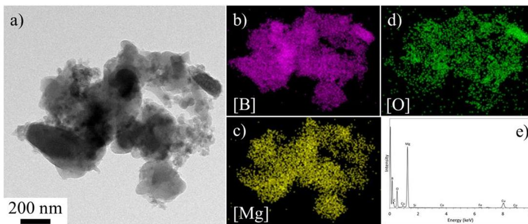
Figure 2: TEM imaging of a magnesium-coated boron nanoparticle agglomerate at a magnification of 15 kX. a) raw TEM image; elemental EDS maps of b) boron, c) magnesium, and d) oxygen; and e) EDS spectrum.
