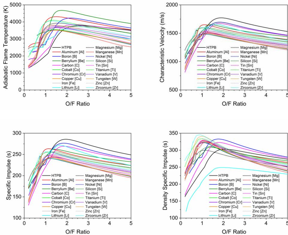
Figure 1: Theoretical performance of HTPB fuel loaded with selected metals at a mass concentration of 50% burning in liquid oxygen (LOX) at a pressure of 1,000 psia (6.89 MPa). Plots depict (top left) adiabatic flame temperature, (top right) characteristic velocity, (bottom left) ideal specific impulse, and (bottom right) ideal density specific impulse.
