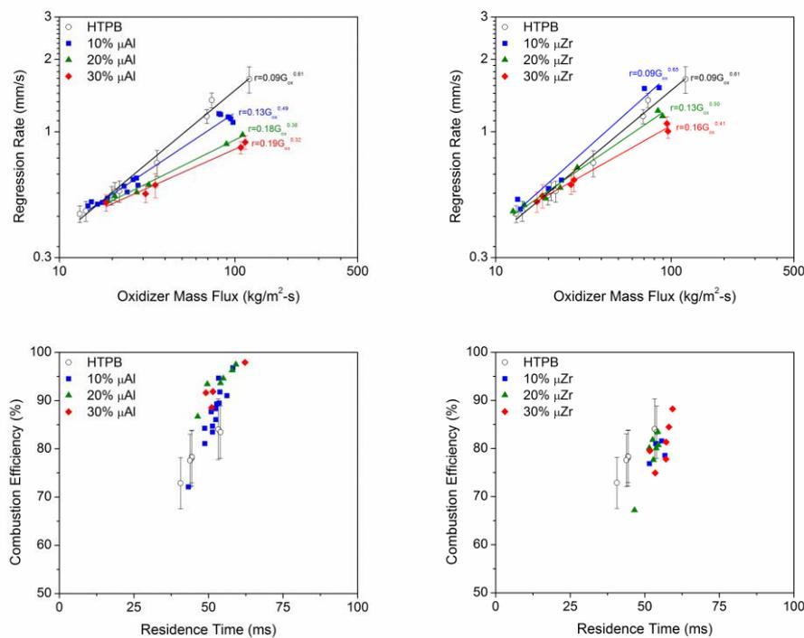
Figure 4: (Top) Regression rates and (bottom) combustion efficiencies for plain HTPB and HTPB loaded with (left) micro-Al and (right) micro-Zr burning in GOX.
