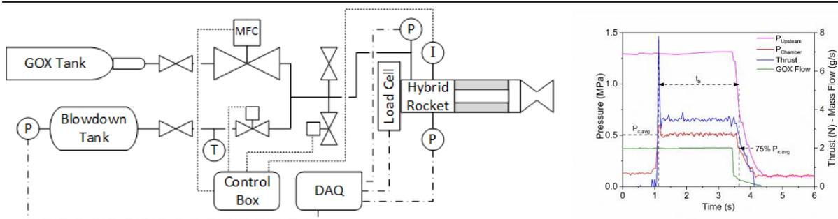
Figure 3: (left) Schematic representation of the hybrid rocket ballistic experiment. (right) Representative transient data traces for plain HTPB burning in GOX at a chamber pressure of approximately 0.52 MPa (75 psia).
