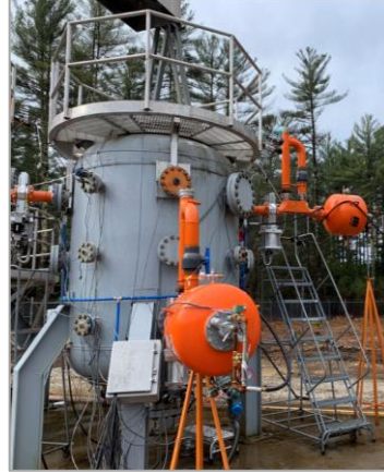
Figure 2: Image of the 8-m 3 test vessel showing the location of two dust injectors.
