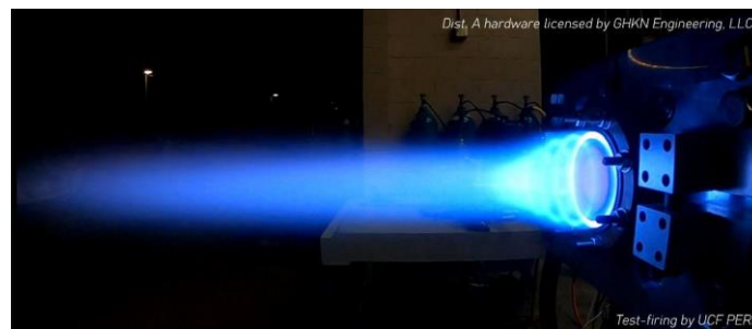
Figure 2: Image of TTS hot-fire operation, showing exhaust plume.
