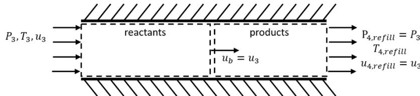
Figure 1: Control volume analysis of the unsteady refilling process.
