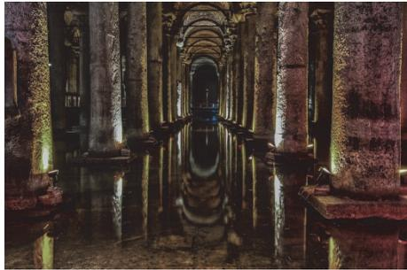
The Ancient Cistern - *Piscina Mirabilis*, partly dug into the tuff, had the capacity of 12,600 cubic meters of water! It was built on a quadrangular plan to obtain four rows of twelve cruciform pillars that divide the interior space into five long and thirteen short naves to support the vault. On the latter it is set the roof terrace paved in terracotta fragments and lime, communicating with the interior by several doors.
