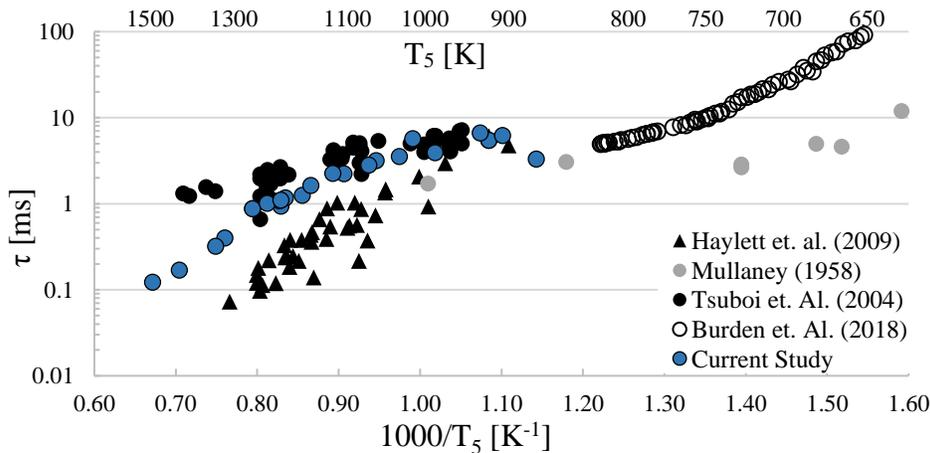
Figure 5: Ignition delay time for diesel spray as a function of reflected temperature for the present study. Results are compared to homogeneous diesel ignition from Haylett et al. [8], shock tube diesel spray from Mullaney [6] and Tsuboi et al. [7], and CVSCC spray measurement from Burden et al. [9].
