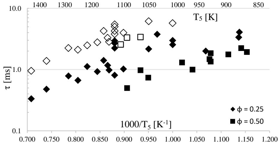
Figure 8: Ignition delay time for premixed methane-argon-oxygen as a function of reflected temperature and reflected shock pressure nominally 10 bar. Solid symbols represent mild ignition and open ones depict strong ignition. The error on the ignition time is 15 microseconds.
