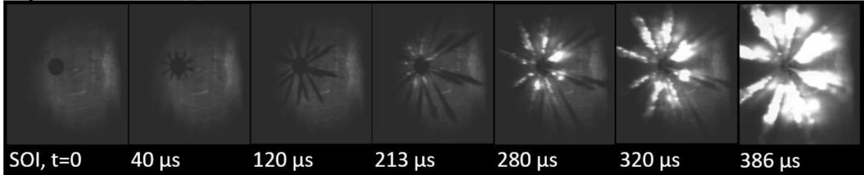
Figure 4: Video frames of ignition location testing for 1300 K, 10 bar initial conditions. It is worth noting the shadow of the spray on the end wall can be seen in addition to the real spray due to the angle of the camera and light source.
