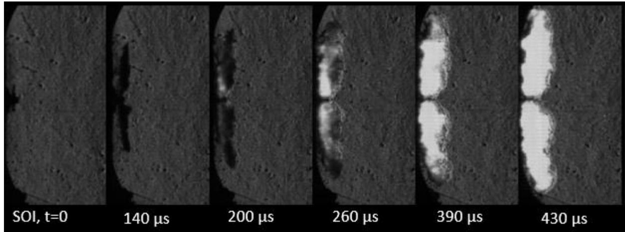
Figure 3: Schlieren images of diesel spray ignition at 10 bar, 1490 K. SOI denotes start of injection.
