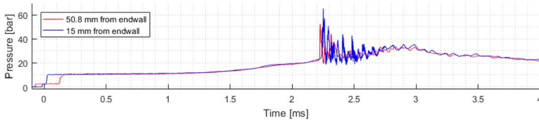
Figure 7: Pressure trace for 2.5% methane at 1130 K, 11 bar.
