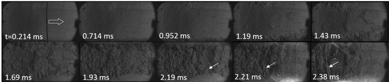
Figure 6: Schlieren images of 2.5% methane ignition at 1130 K, 11 bar. Time-zero corresponds to time of shock wave reflection.
