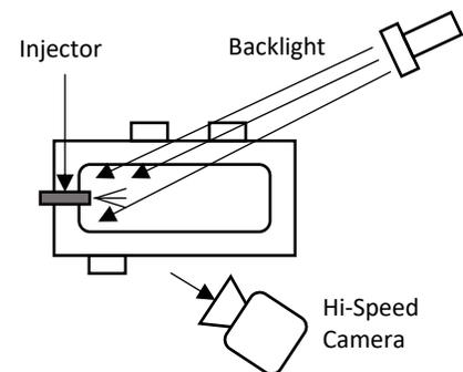
Figure 2: Schematic of the optical section in the regular photography configuration.
