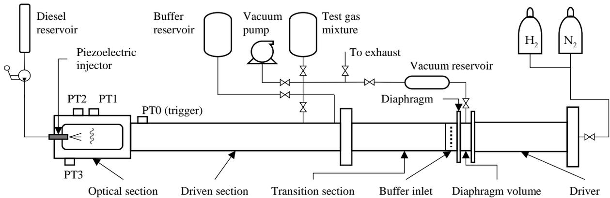
Figure 1: Experimental schematic of the shock tube, illustrating the optical section, buffer inlet and injector assembly.
