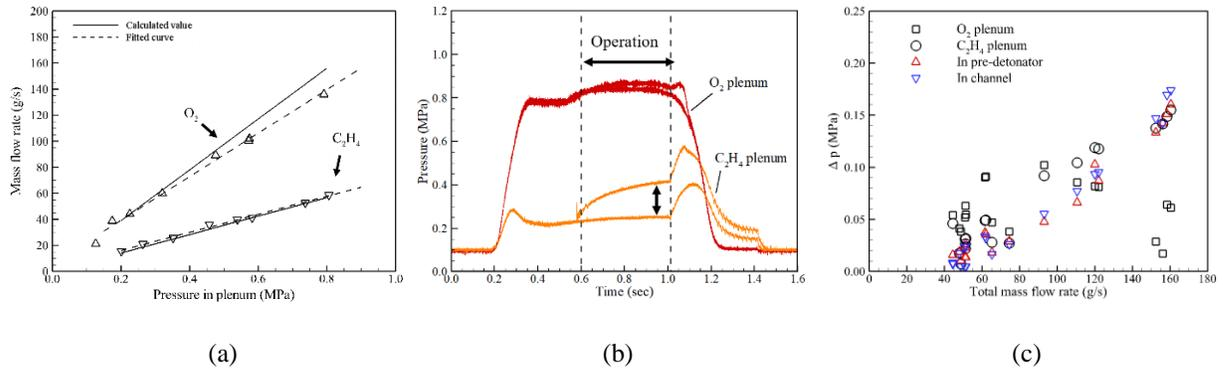
Figure 3. Measured operational flow parameters: (a) mass flow rate,  $\dot{m}$ , (b) pressure variation in plenum and (c) pressure differences at flow locations.
