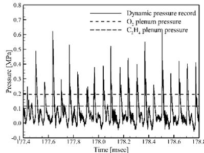
Figure 4. Pressure record of the rotating detonation in combustion channel at  $\dot{m} = 48.6$  g/s,  $\Phi = 0.91$
