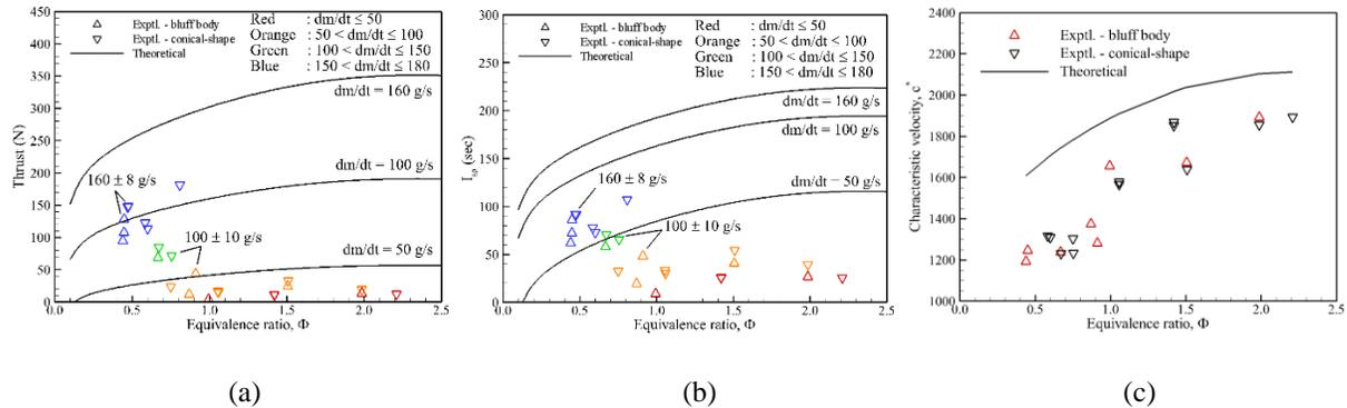
Figure 6. Performance parameters with respect to the equivalence ratio,  $\Phi$ : (a) thrust,  $F$ , (b) specific impulse,  $I_{sp}$ , and (c) characteristic velocity,  $c^*$
