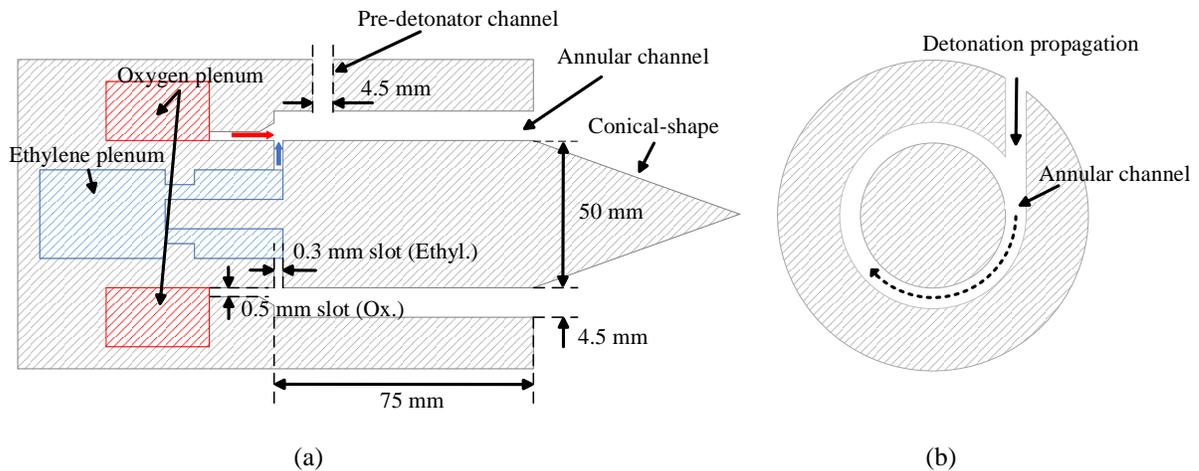
Figure 1. Schematic of the RDE: (a) sectional side view and (b) sectional front view
