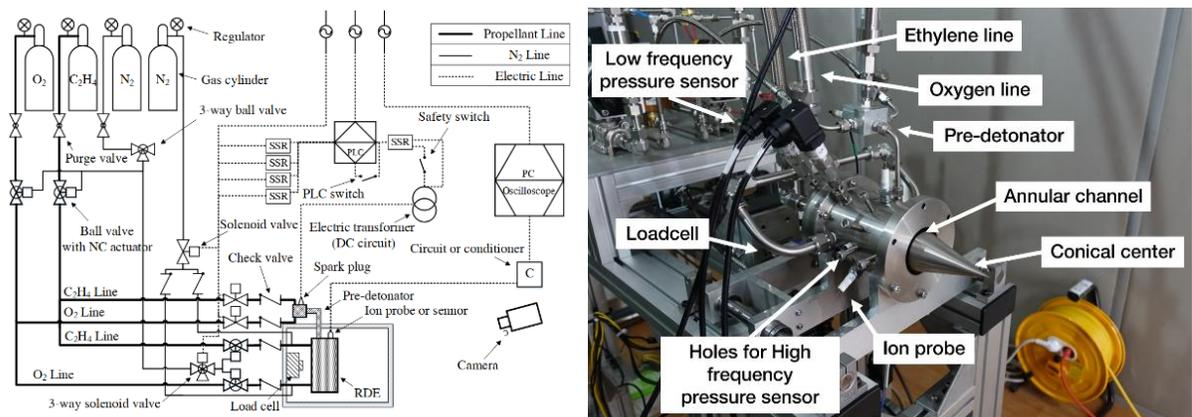
Figure 2. Schematic of propellant supply and control system (left) and a picture of the experimental setup (right)
