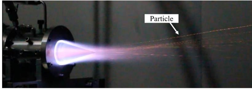
Figure 5. Direct picture of RDE plume on ablation phenomenon at  $\dot{m} = 163.0$  g/s,  $\Phi = 0.47$  (3,840x2,160 resolution using Sony RX-100M5 camera)
