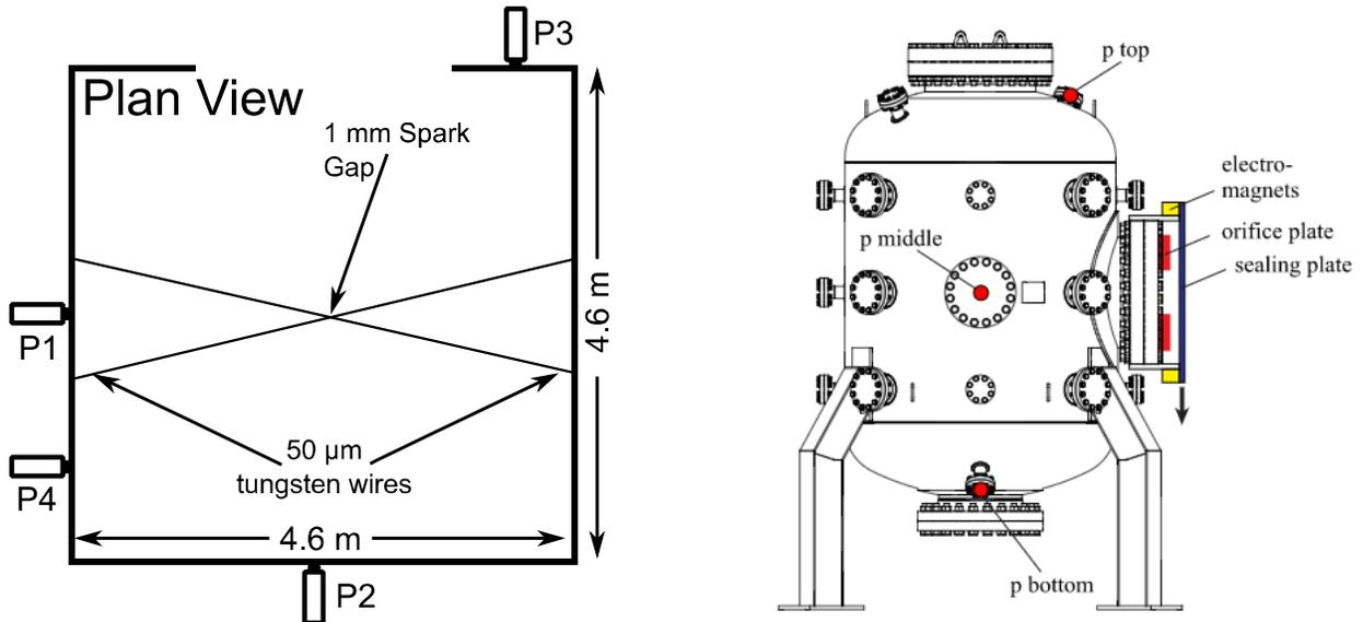
Figure 1. Diagrams of the 64 m<sup>3</sup> chamber [7, 8, 9] (left) and the 8 m<sup>3</sup> vessel [10] (right)
