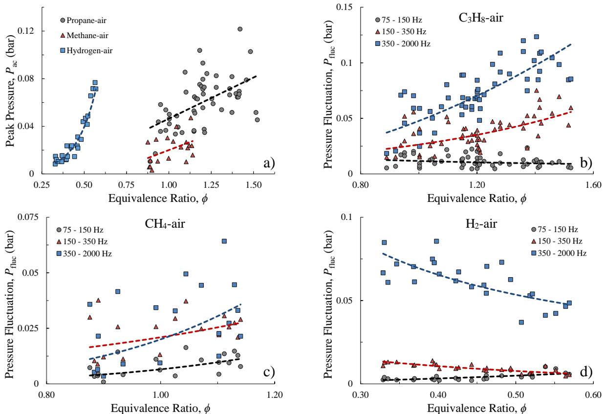
Figure 4. Plots showing a) the peak mean pressure associated with flame-acoustic instabilities in the 64 m<sup>3</sup> chamber, and the peak pressure fluctuations, for three pressure ranges, in b) propane, c) methane, and d) hydrogen mixtures.
