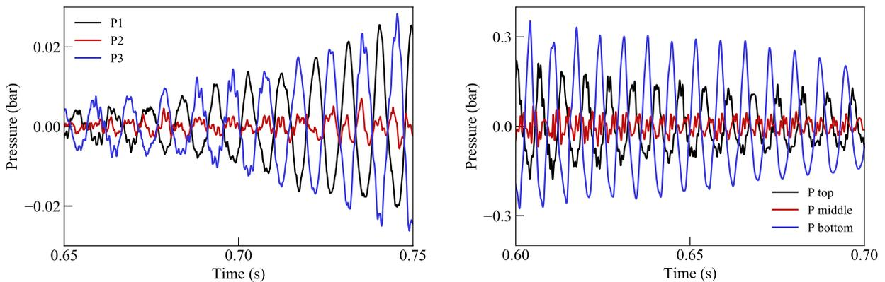
Figure 3. Example plots showing the presence of a 100 Hz standing wave in 64 m<sup>3</sup> chamber and a 150 Hz standing wave in the 8 m<sup>3</sup> vessel.
