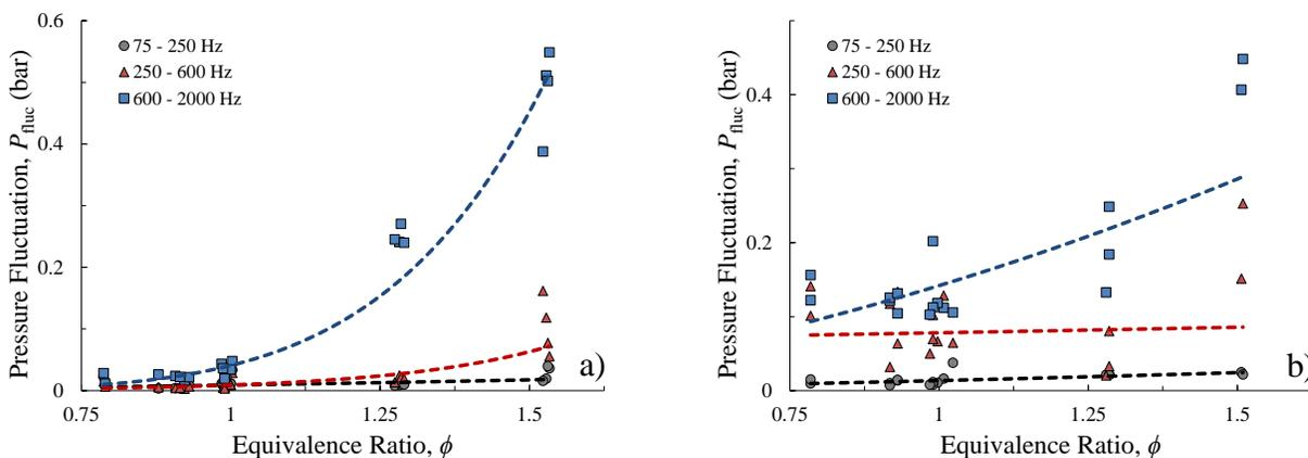
Figure 5. Peak pressure fluctuations, for propane-air mixtures, in a) confined and b) vented, 8 m<sup>3</sup> vessel.
