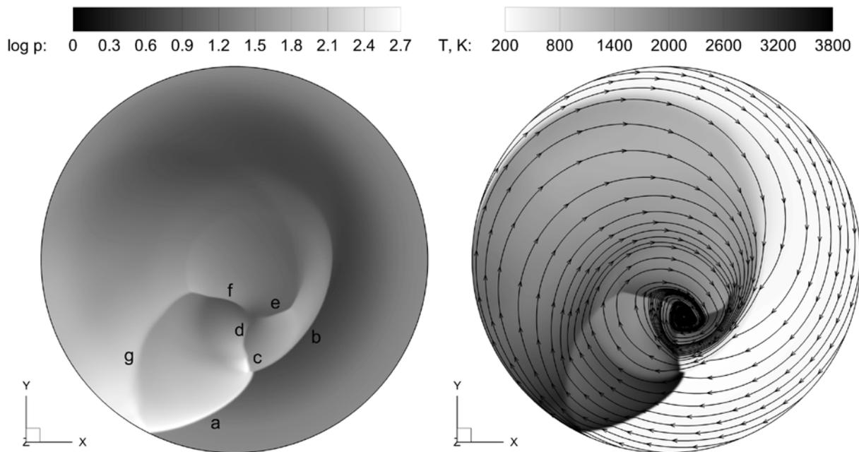
Figure 3. Pressure field (left) and temperature field (right) in the exponential scale for steady counterclockwise rotating detonation. The streamlines on the right figure are presented in the coordinate system rotating with the wave
