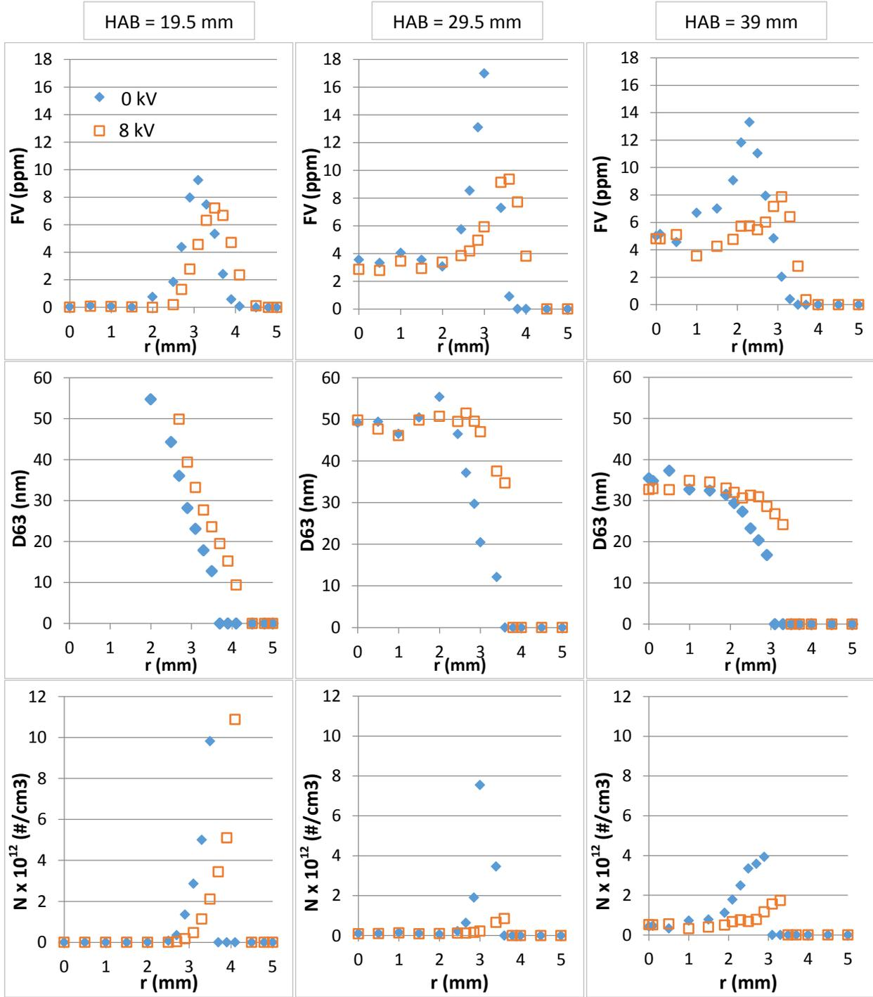
Figure 2. Soot volume fraction  $f_v$ , particle mean diameter  $D_{63}$  and number concentration  $N$  along the flame radius at 19.5, 29.5 and 39 mm HAB positions.
