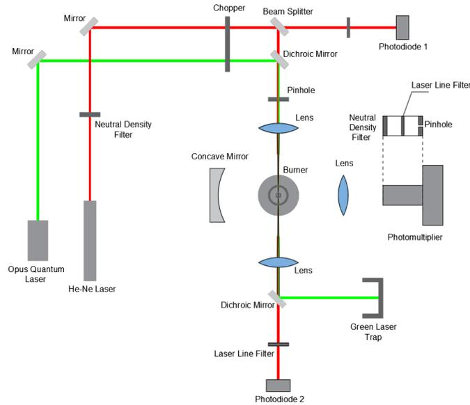
Figure 1. Schematic of the optical setup
