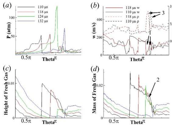
Figure 4 Quantities on the  $r = R_{outer}$  slice and on the headwall. (a) Pressure; (b) axial component of velocity and density; (c) height of fresh gas layer; (d) mass of fresh gas.
