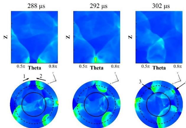
Figure 2 Unwrapped maps and bottom views of pressure contours at  $t = 288 \mu\text{s}$ ,  $292 \mu\text{s}$  and  $302 \mu\text{s}$ . 1-Clockwise wave; 2-counterclockwise wave; 3-remaining detonation wave; 4-abscising part.
