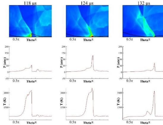
Figure 3 Detonation/shock collision process on the  $r = R_{outer}$  slice. (a) Unwrapped maps of pressure contours of this slice. (b) Pressure on the headwall. (c) Temperature on the headwall.
