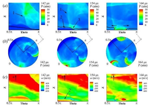
Figure 7 Contours at  $t = 142 \mu\text{s}$ ,  $154 \mu\text{s}$  and  $164 \mu\text{s}$ , respectively. (a) Unwrapped maps of pressure contours; (b) Bottom views of pressure contours; (c) Unwrapped maps of axial velocity contours. Lines in (a) and (c) separates fresh gas and combustion products. 1-Shock wave; 2-surface of pressure discontinuity; 3-intersection of 1 and 2.
