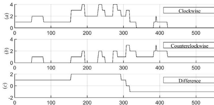
Figure 8 Number of detonation waves. (a) Clockwise waves (b) counterclockwise waves and (c) clockwise waves minus counterclockwise waves.
