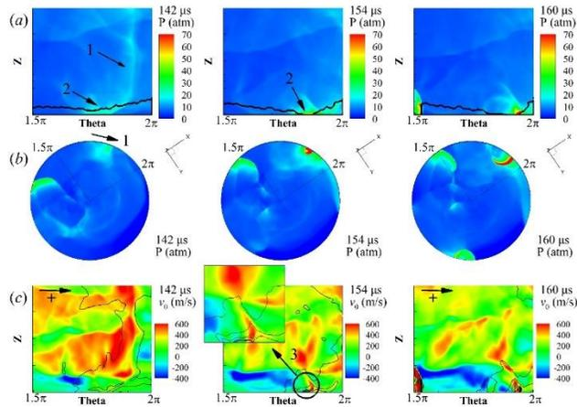
Figure 6 Contours at  $t = 142 \mu\text{s}$ ,  $154 \mu\text{s}$  and  $160 \mu\text{s}$ , respectively. (a) Unwrapped maps of pressure contours with lines separating fresh gas and combustion products; (b) Bottom views of pressure contours; (c) Unwrapped maps of circumferential velocity contours with lines of pressure.
