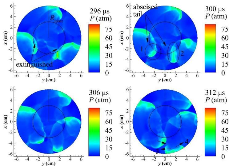
Figure 5 Bottom views of pressure contours at  $t = 296 \mu s$ ,  $300 \mu s$ ,  $306 \mu s$  and  $312 \mu s$ , respectively.
