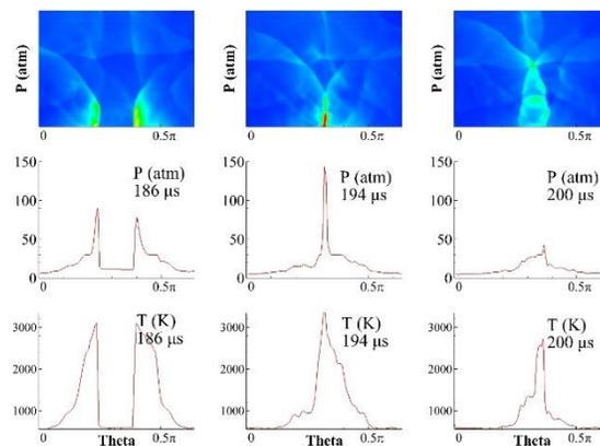
Figure 1 Detonation/detonation collision on the  $r = R_{\text{outer}}$  slice. (a) Unwrapped maps of pressure contours. (b) Pressure distribution on the headwall. (c) Temperature distribution on the headwall.
