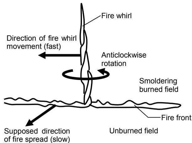
Figure 1. Schematic diagram of a moving fire whirl over a line fire that was observed in Brazil in 2010
