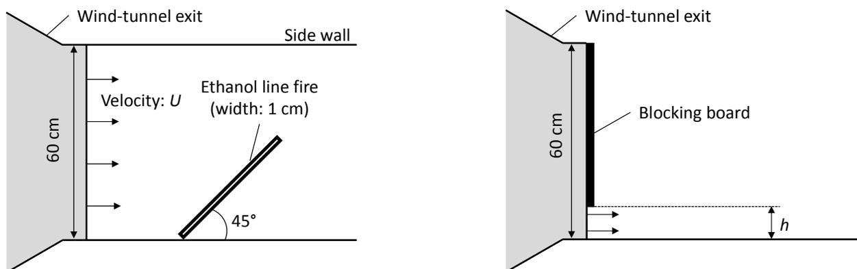
Figure 2. Schematic diagram of the experimental configuration. Left: a top view; right: a side view
