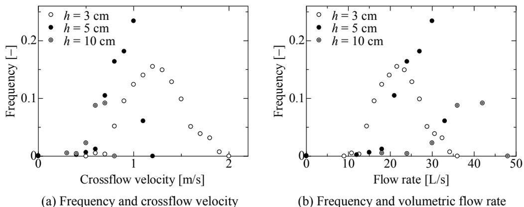
Figure 5. Frequency of fire-whirl formation at three different values of opening-height  $h$  of wind-tunnel exit
