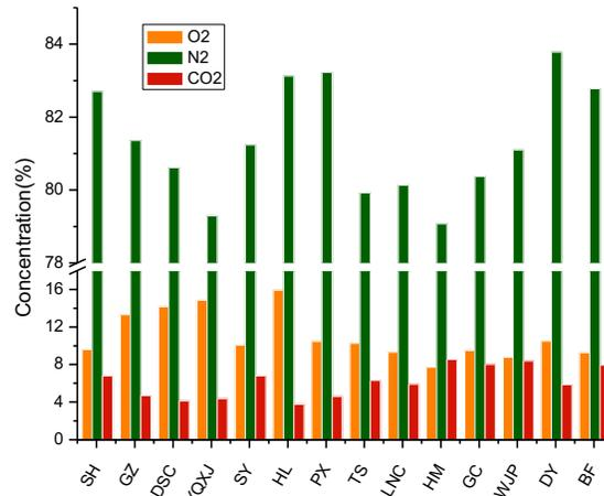
Figure 2: Concentration of O<sub>2</sub>, N<sub>2</sub> and CO<sub>2</sub> in post-explosion gas
