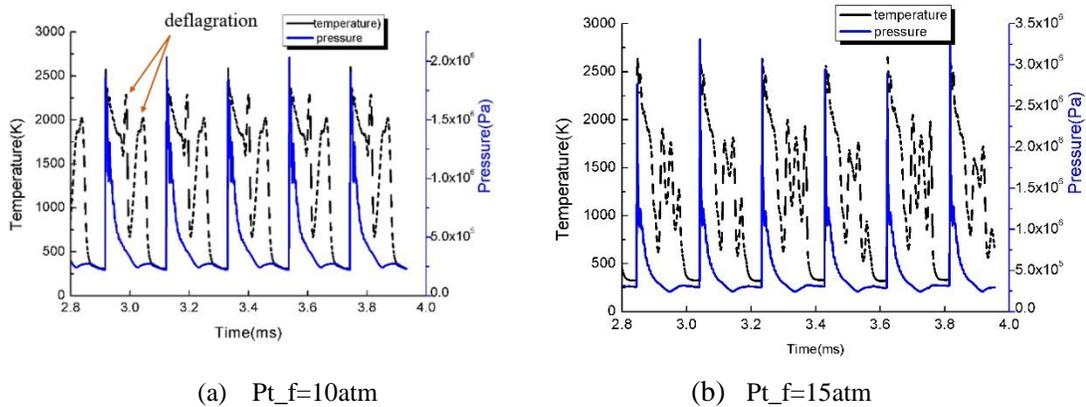
Figure 4. Detonation parameter variations with time
