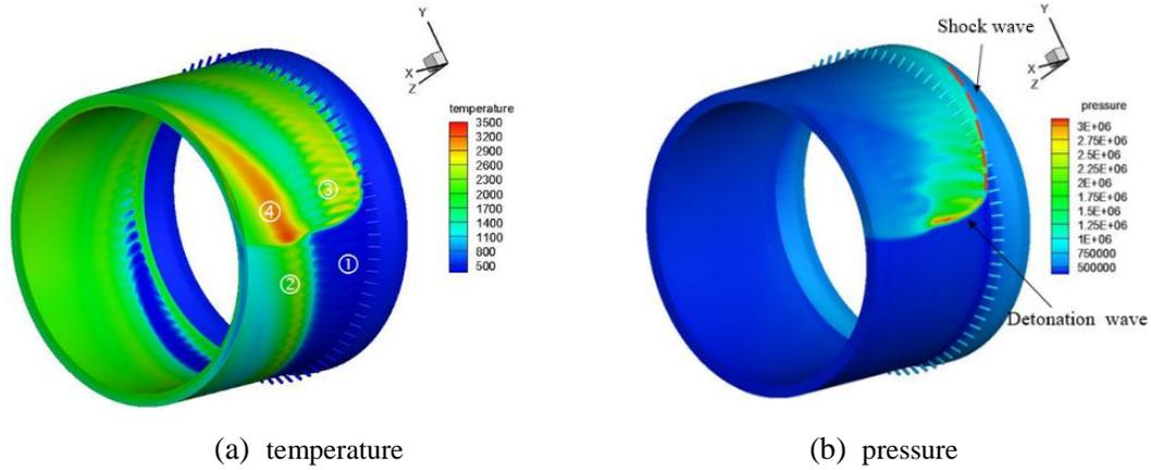
Figure 3. Instantaneous parameter distribution near the external wall of RDC
