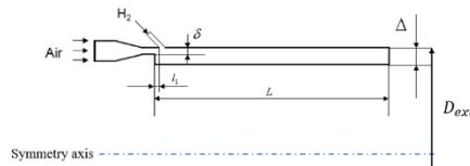
Figure 1. Rotating detonation combustor model
