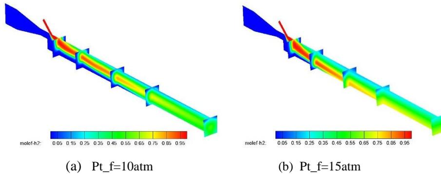
Figure 2. Species fraction distribution of hydrogen at different injection pressures
