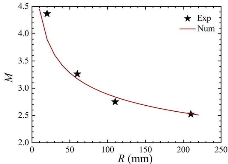
Figure 6. Numerical results (Num) compared with experiment results (Exp) of  $M$ - $R$  relation in the converging part
