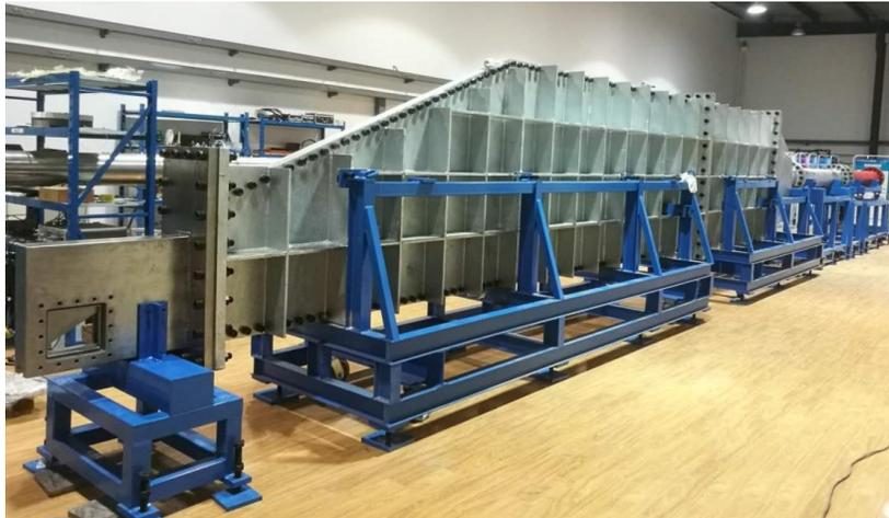
Figure 4. Photograph of the shock tube
