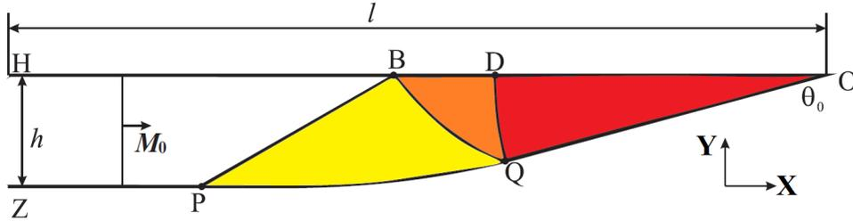
Figure 1. The schematic of the wall profile.  $h$ : the shock tube height;  $M_0$ : the Mach number of the incident planar shock;  $\theta_0$ : the converging angle;  $l$ : the distance between the point O and H; ZHBP: uniform zone; PBQ: simple-wave zone; BQD: double-wave zone; DOQ: converging part
