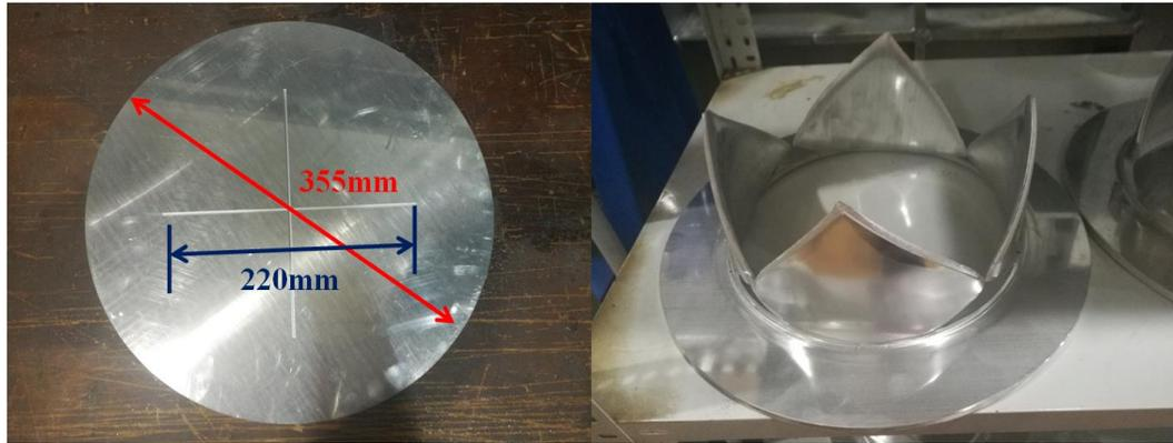
Figure 5. Left: initial diaphragm; right: ruptured diaphragm
