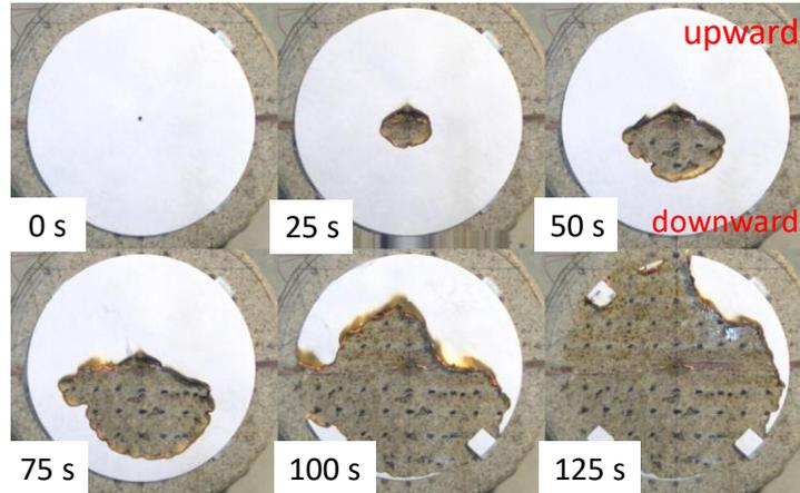
Figure 1. Flame spread when the Terada phenomenon occurs ( $d_L = 3$  mm,  $\theta = 35^\circ$ )
