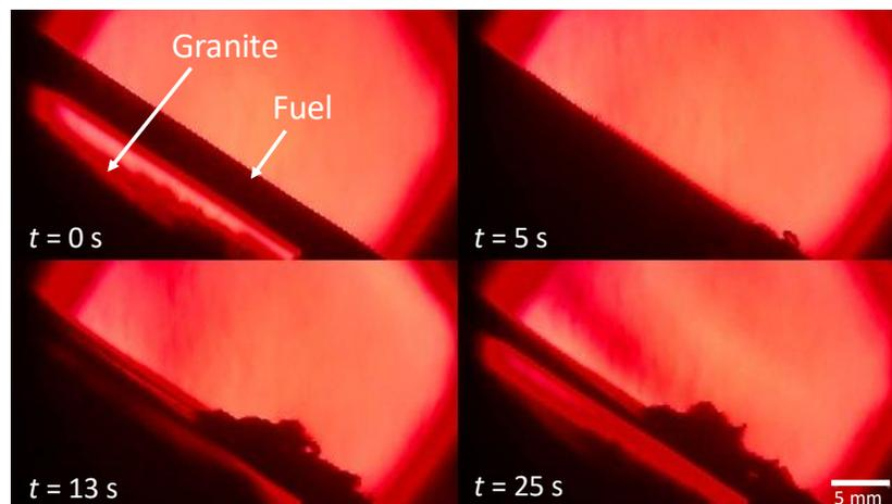
Figure 6. Vicinity of the filter paper surface in the upward slope direction from the ignition point ( $d_L = 3 \text{ mm}$ ,  $\theta = 35^\circ$ )
